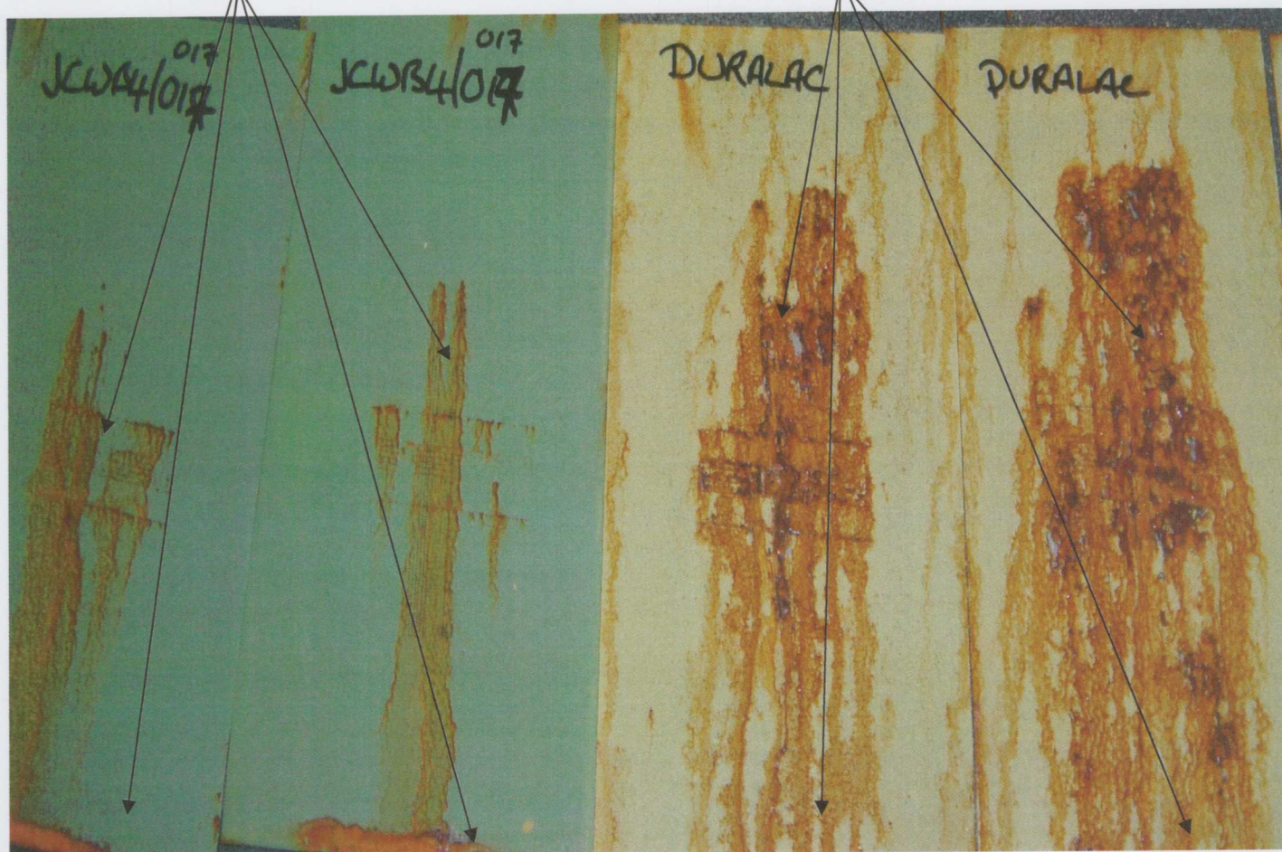
Corrosion confined to cross hatch area
