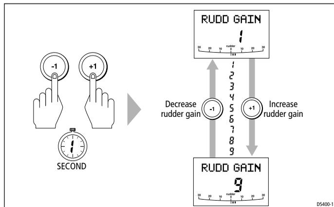
On Type 150/400 (non-GyroPlus) and Type 100/300 systems, you can make temporary adjustments to rudder gain to change the autopilot's steering characteristics. Rudder gain is a measure of how much helm the autopilot will apply to correct course errors:
