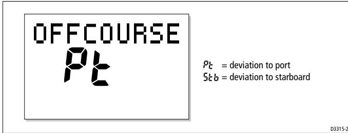
The ST6001+ activates the OFF COURSE warning when the boat has been off course from the locked heading by more than the specified angle\* for longer than 20 seconds. It shows whether the deviation is to port or starboard.
