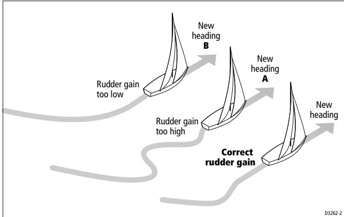
To adjust the rudder gain:
