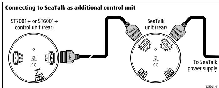
We supply the ST6001+ with a 9 m (29 ft 6 in) SeaTalk cable as standard. Depending on your installation, you may need to obtain alternative or additional SeaTalk cables (as shown in the following illustration).
