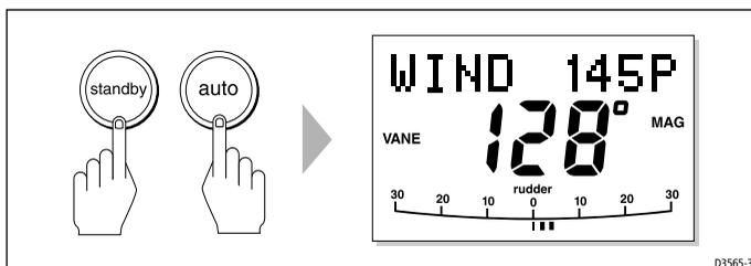
The autopilot will then adjust the boat's heading to maintain the locked wind angle.
