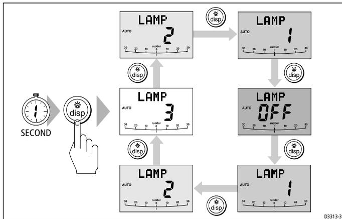
3. The display automatically returns to the previous mode if you do not press a key for 10 seconds:
