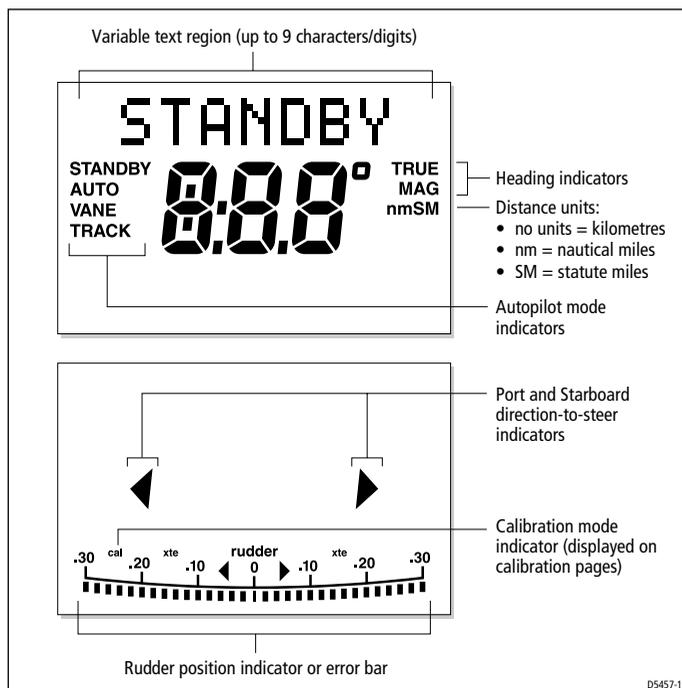
The bar graph at the bottom of the screen is normally a rudder position indicator. This indicates the current position of the rudder, as measured by the rudder position sensor.
