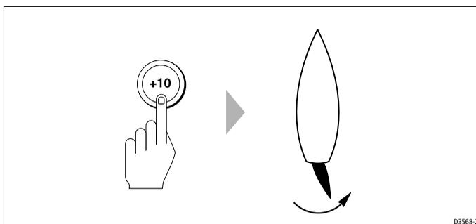
If the rudder moves to port or the rudder drives hardover:
