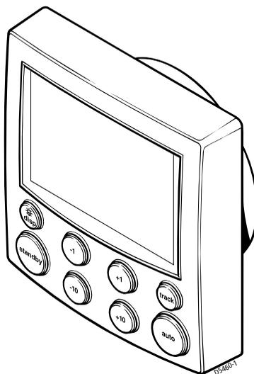
The Raymarine ST6001 Plus (ST6001+) is a SeaTalk<sup>®</sup> compatible autopilot control unit. It is designed as the main control unit for Raymarine Type 150, 150G, 400 and 400G course computers.
