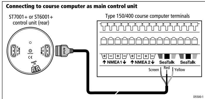
**Note:** If you are connecting the ST6001+ to a course computer autopilot system that includes other control units, refer to the information contained in the Autopilot System Installation Guide.
