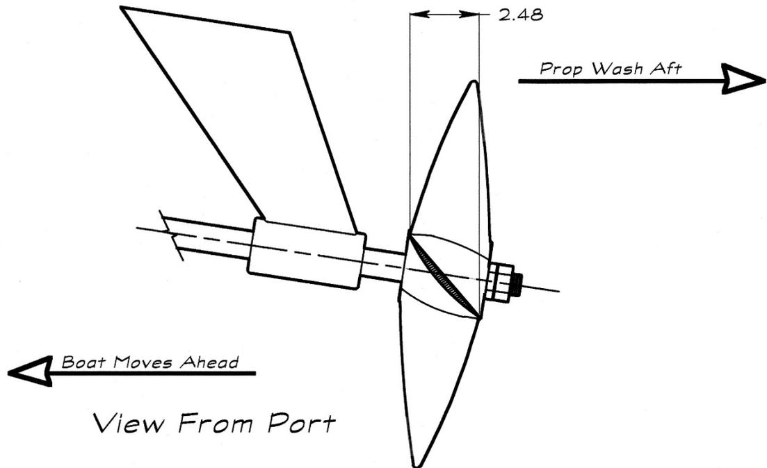
Side Thrust From Shaft Angle
