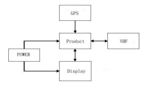
Figure 2 Connection Diagram
