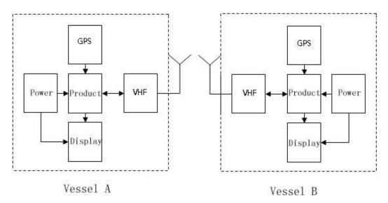
Figure 1 AIS Class-B AIS system Block Diagram
