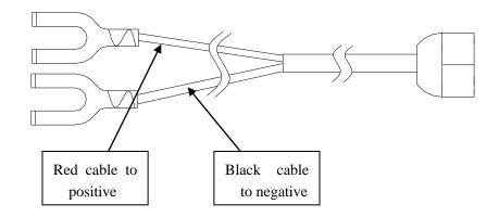
Figure 4 DC interface diagram
