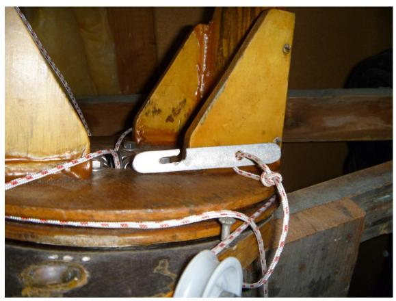
One of the two aluminium hooks which made clipping the steering lines on easy.
