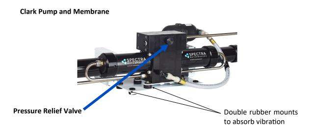
This module must be installed in an area that maintains a temperature below 113°F (45°C). It may be placed as high in the boat as you desire, and mounted in any position, even upside down. Make sure that the area around and under the pump does not have any water sensitive equipment, as water will be spilled during any repairs or if a leak occurs. Allow for easy access to the pressure relief valve.
