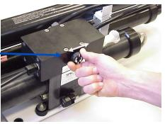
feel more slippery, than water. Stop the pump by moving the switch back to 'RUN AUTO'. Add more propylene glycol to the intake bucket if necessary.
