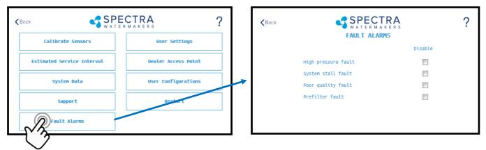
CAUTION! Never disable a Fault Alarm without being certain that the issue is with a bad sensor. Disabling a fault and running the system can cause serious damage or injury.
