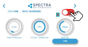
**Note:** The system will automatically drop to Low Mode when it senses high feed pressure, or dirty pre-filters.
