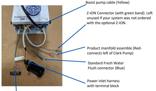
Tank Full Switch Terminal Block, Green + Orange
