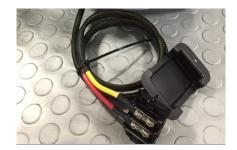
Mount the main power terminal block in a junction box or on a bulkhead adjacent to the feed pump module. Make sure that this is a dry location well above bilge level and not subject to water spray. **Be sure to install the terminal block cover.**
