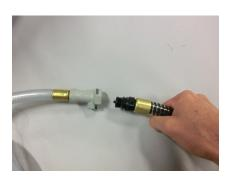
Attaching intake service hose to the hose connecting to the sea strainer.
