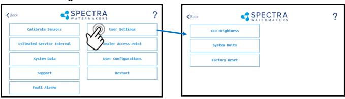
LCD Brightness: Set brightness of the hardwired display(s) from 10—100%
