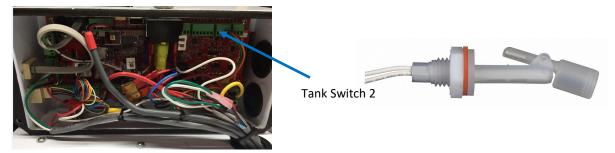
The float switch must be connected to the Tank Switch 2 terminals on the Spectra Connect control board at the Feed Pump Module. There is no polarity.
