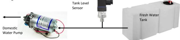
Route the 3 conductor cable back to the Spectra Connect control board at the feed pump module. Extend the wires as necessary. *If you must extend the wires beyond 50' contact the factory to ensure proper operation.*
