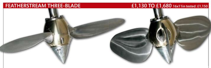
Made in England for the past 18 months, this is a three-blade feathering unit with a bronze boss and stainless steel blades. The pitch of the blades can be adjusted externally, and can be different for ahead and astern. The blades swivel 180° to present the same leading edge in ahead
