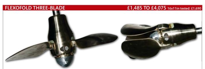
Made in Denmark for the past 12 years, the Flexofold is an all-bronze folding unit, with blades fixed by stainless steel pins, and the anode, which covers the gearing, cleverly enclosed by the folded blades. On test, it gave the equal highest forward thrust of all props, and highest top speed. It also had one of the lowest side-thrusts. Going astern, its performance was the best of all the folding propellers.
