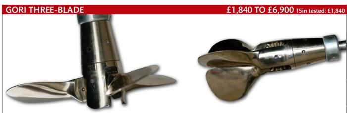
Another of the earliest folding designs, the Gori propellers have been made in Denmark since 1975, in two and three-blade versions, but the company only recommended the three-blade for this boat. Gori also makes a racing two-blade version. The blades have a three-way gearing
