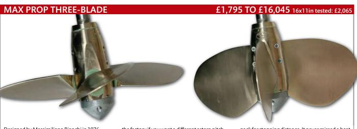
Designed by Massimiliano Bianchi in 1976, the Max Prop was one of the first of the new generation of props. Boss and blades are bronze, and the pitch can be set as you assemble it, or by
