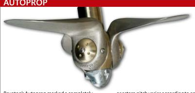
Brunton's Autoprop marked a completely different approach to feathering props when it was brought out in 1987. The three blades rotate independently, going from fully feathered while sailing, or in neutral, to fully twisted under power. The difference is that when you go into gear, the amount they rotate depends on engine speed and loading. Thus the ahead
