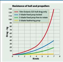
At 5 knots, a fixed three-blade prop with its shaft locked creates almost half as much drag as the entire hull. The drag can be halved by allowing the prop to spin, but the gearbox may suffer. By contrast, the drag of a feathering prop is negligible, and the drag of a folding prop is too small to plot on a graph of this scale.
