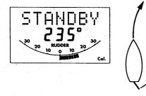
If the display moves in the opposite direction the red and green wires of the rudder reference transducer should be reversed.
