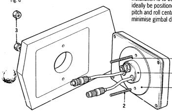
Pass the cable tails through the central hole and secure the instrument with the thumb nuts provided 3. (A sealing gasket 4 is already attached to the back cover).
