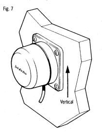
Correct positioning of the fluxgate is crucial if ultimate performance from the autopilot installation is to be achieved. The fluxgate should ideally be positioned as near as possible to the pitch and roll centre of the vessel in order to minimise gimbal disturbance (Fig. 8).
