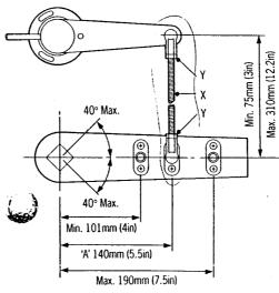
With the rudder amidships, the rudder reference arm should be opposite the cable entry and at 90 deg. to the connecting bar. Minor adjustment can be made by slackening off the 3 securing screws and rotating the transducer body.
