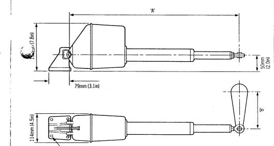
4 off Fixing holes suitable for 10 mm (0.4in) bolts.
