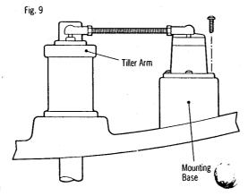
The rudder reference unit has a built in spring to remove any free play in the linkage to the tiller. This gives very precise rudder position. The rudder reference arm movement is limited to  $\pm$  60 deg. Care must be taken during installation to ensure the rudder reference arm is opposite the cable entry when the rudder is amidships. Failure to do this could result in damage if the rudder reference arm is driven onto its end stops by the steering system (Fig. 10).
