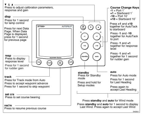
Note: The up arrow, down arrow, **resp, track, set crs** and **res'm** keys can also be used to set up and control groups of Autohelm ST60 and ST80 instruments (see Section 2.8, Remotely Controlling ST60 and ST80 Instruments and Section 4.3, Setting Up For ST60 and ST80 Remote Control).
