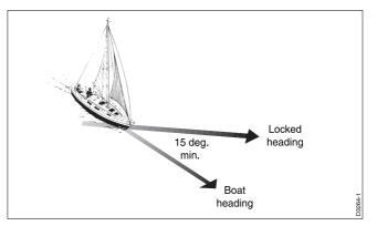
The value must be within the range 15 to  $40^\circ,$  and can be adjusted in  $1^\circ$  steps.
