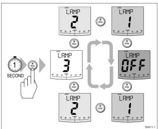
Press the **disp** key the necessary number of times to cycle to the required illumination setting. The settings are LAMP 3, LAMP 2, LAMP 1, LAMP OFF, LAMP 1, LAMP 2, LAMP 3 etc, with LAMP 3 being the brightest setting.
