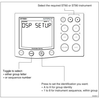
When setting up an instrument group, you need to understand the indications which show when an instrument is selected. This depends on instrument type as follows:
