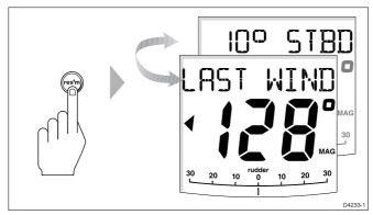
The LAST WIND text alternates with the previous wind angle and direction (PORT or STBD). The previous locked heading is displayed, with an indicator to show you the direction in which the vessel will turn.
