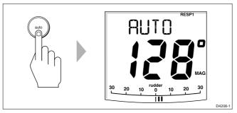
· In Auto mode, the display shows the locked autopilot heading.
