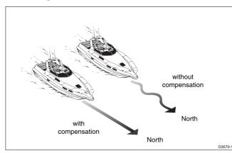
The AutoAdapt feature allows the Course Computer to compensate for heading errors at higher latitudes, which are caused by the increasing dip of the earth's magnetic field. The increased dip has the effect of amplifying rudder response on northerly headings in the northern hemisphere, and on southerly headings in the southern hemisphere.
