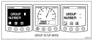
5. Use the ST7000 Plus to allocate a group letter and sequence number to the selected instrument. To do this, use the **track** key to toggle between group letter and sequence number, and the **set crs** key to set the identifying character. When the instrument has been properly identified it should display its group letter and sequence number, e.g. A2.
