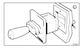
The Joystick is supplied with 26ft (8m) of cable which should be connected to the course computer as shown.
