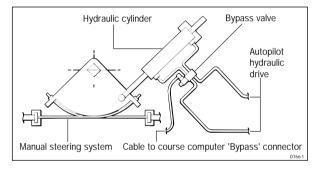
*Note:* The bypass valve voltage must be matched to the course computer supply voltage, i.e. 12V or 24V.
