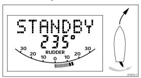
If the display moves to the left the red and green wires from the rudder reference transducer must be reversed.
