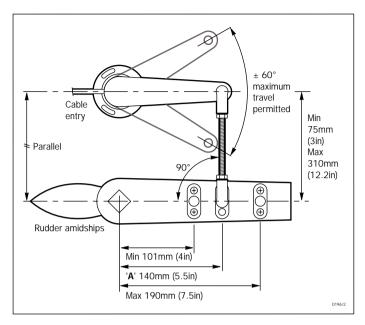
It is important to ensure that the dimensions (set out above) are within the set limits and that the tiller and rudder reference arms are parallel to each other.
