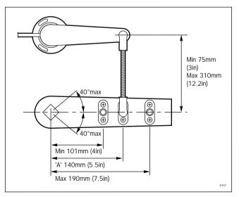
With the rudder amidships, the rudder reference arm should be opposite the point of cable entry and at 90 degrees to the connecting bar. Minor adjustments can be made by loosening the 3 securing screws and rotating the transducer body.
