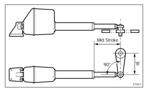
**Caution:** The linear drive system can exert a thrust of over 1000lb. (450Kg). The steering gear manufacturer must be consulted if any doubt exists about the strength of the existing tiller arm or rudder quadrant.
