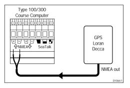
Connect the NMEA input on the radar etc. to the NMEA output terminals on the course computer.
