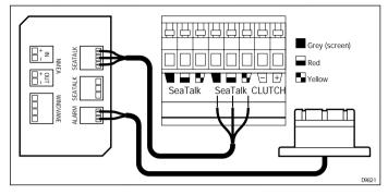
Connect the NMEA interface to the alarm and course computer as shown.
