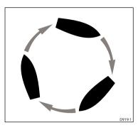
Keep turning until the display changes to show the amount of deviation the autopilot has corrected. This can take up to 2 full turns depending on the amount of deviation found.
