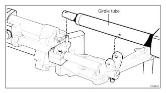
Carefully twist and lower the actuator in to the girdle support bracket until the spring pin locates into the opposite side of the girdle tube.
