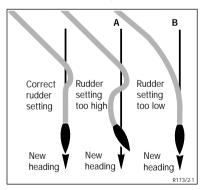
*Note:* Once the optimum setting has been found, the default calibration setting for rudder gain should be changed.
