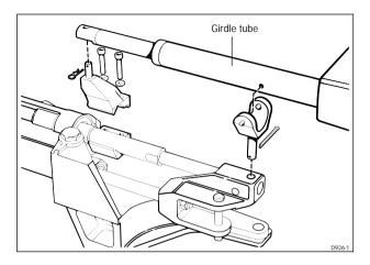
7. Carefully twist and lower the actuator into the girdle support bracket until the spring pin locates into the opposite side of the girdle tube.
