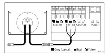
If the vessel is already fitted with Autohelm instrumentation, this should be connected to the course computer as shown, using one of the standard SeaTalk interface cables. The course computer will then supply power for the complete system.
