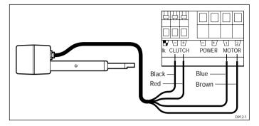
labelled clutch and motor as shown.
