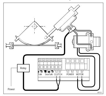
*Note:* A 5 amp relay should be used to energise the bypass valve. The relay should have a 12V coil (taking less than 500ma) and be driven by the clutch output on the course computer connector.
