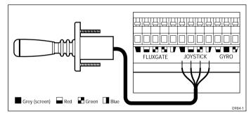
Note: Only one joystick can be connected.
