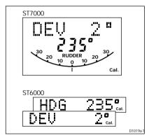
*Note:* If the deviation exceeds 15 degrees, you should relocate the fluxgate compass.
