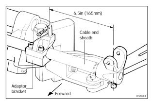
*Note:* The securing bolts must be on the front or bow of the boat side cable end sheath. Also, the bracket should be positioned 6.5in (165mm) from the girdle support bracket.
