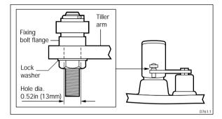
The mounting bracket should be bolted to a substantial frame member.
