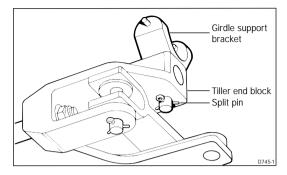
2. Secure the assembly with the split pin (supplied).
