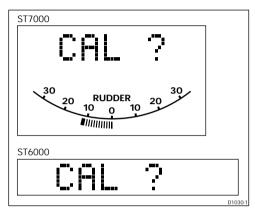
• Press and hold **Track** and **Display** for a further 2 seconds to access the following display.
