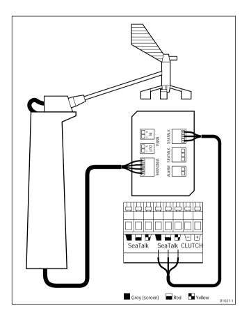
*Note:* The yellow connection from the mast head transducer is not connected at the NMEA interface.
