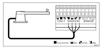
2. Connect to the rudder reference terminals on the course computer.
