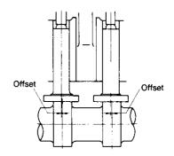
NOTE: When removing tappets, be sure to keep them separate for each cylinder and intake/exhaust valve.
