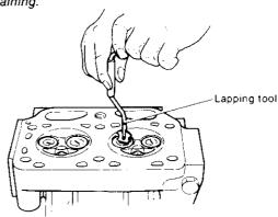
NOTE: 1. Insert adjusting shims between the valve spring and cylinder head when seats have been refinished with a seat grinder.
