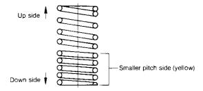
NOTE: The pitch of the valve spring is not even. The side with the smaller pitch (yellow) should face down (cylinder head) when assembled.
