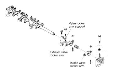
(1) Valve arm shaft and valve arm bushing
