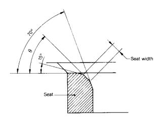
(2) Knead valve compound with oil and finish the valve seat with a lapping tool.
