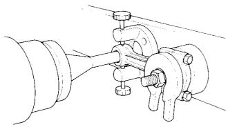
NOTE: Attach the bushing to the piston pin so that a pin, coated with engine oil can be pushed into position with your thumb.
