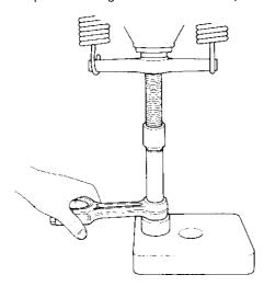
NOTE: Force the piston pin bushing into position so that its oil hole coincides with the hole on the small end of the connecting rod.
