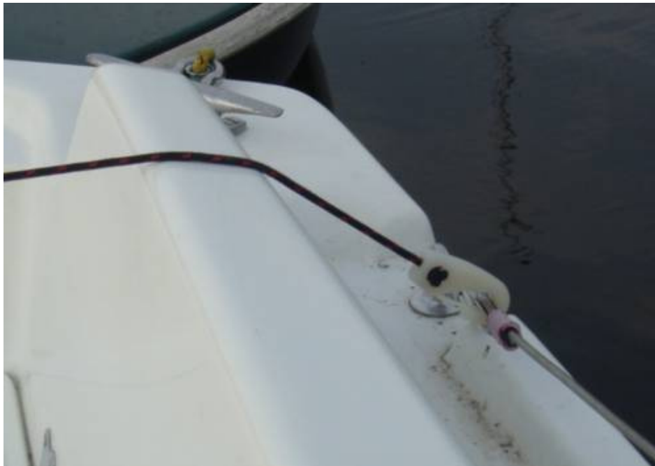
Transverse sheet horse clipped to the aft guardrail eye on each side
