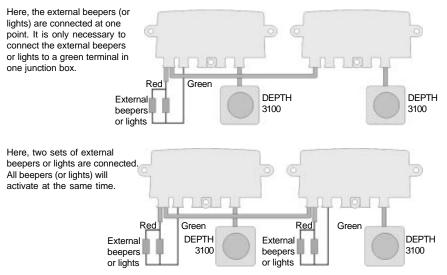
Important: Ensure wires are stripped and tinned.
