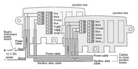
Note: the 10 m (33 ft) NAVMAN power and NavBus data cables can be cut if required.
