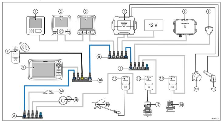
Note: The system allows up to 3 instrument displays to be daisy chained as shown in the example above.
