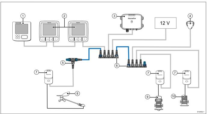
**Note:** The i70 has the capability of connecting to SeaTalk or SeaTalkng networks however if data bridging is required a SeaTalk to SeaTalkng converter is needed.
