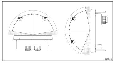
**Note:** The angles are provided for a contrast ratio of equal to or greater than 10.
