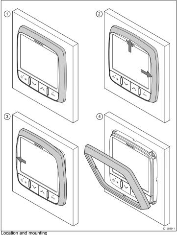
**Important:** Use care when removing the bezel. Do not use any tools to lever the bezel, doing so may cause damage.
