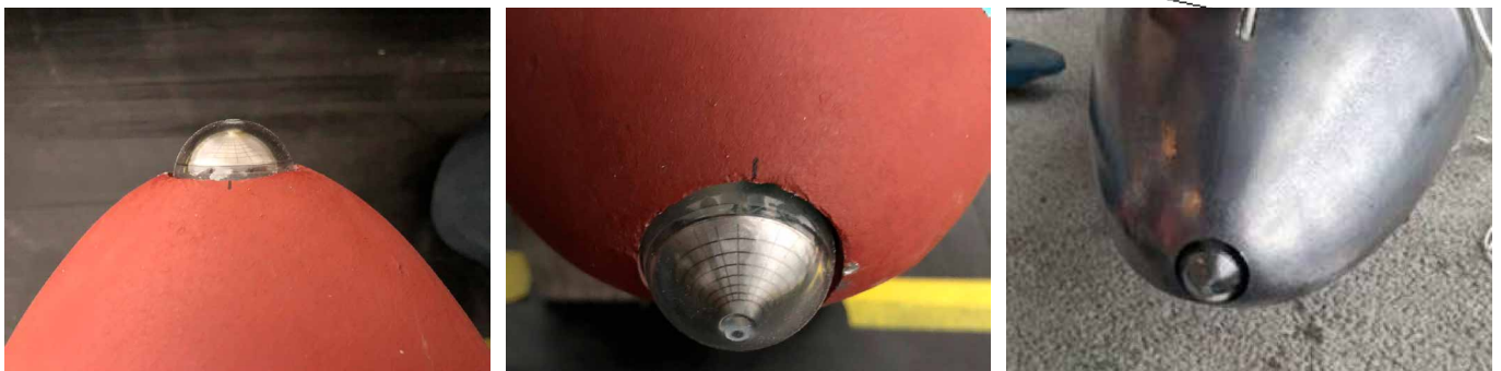
WhaleShield installed in keel bulb, prior to bonding in place.
