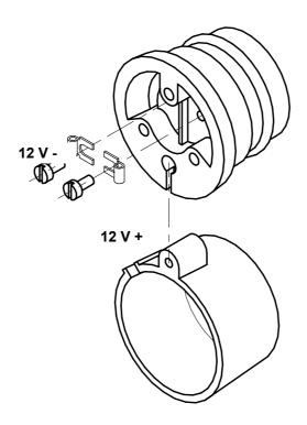
AFIN D'ÉVITER TOUT PROBLÈME D'OXYDATION PAR ELECTROLYSE, IL EST RECOMMANDÉ DE NE PAS LAISSSER LA PRISE SOUS TENSION LORSQUE LE PILOTE N'EST PAS EN FONCTIONNEMENT.
