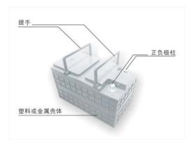
提手: Handle 正负极柱: Positive and negative terminal 塑料或金属壳体: Plastic or metal case
