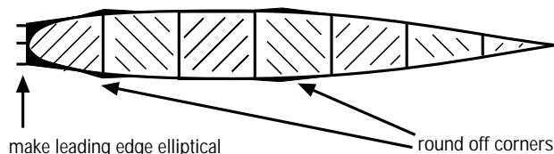
Leave 1mm width on the trailing edge of sheathed boards and up to 3-4mm on boards not sheathed.
