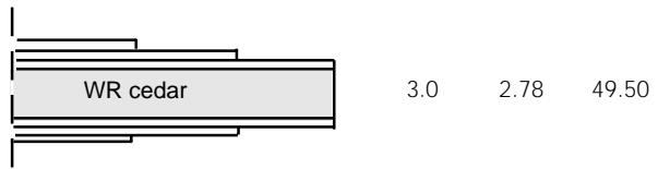
Example 5 - WR Cedar + 4 layers UD carbon to 40%, 70%, 2x 100% span respectively
