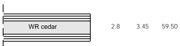
Example 4 - WR Cedar + 3 layers UD carbon to 40%, 70%, 100% span respectively
