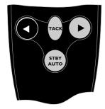
Fig 3 - Remote steering to Port in Standby mode
