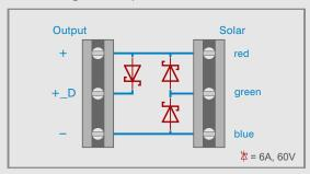
24V: Serial connection of 24V solar modules
