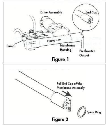
**NOTE:** End Caps may not come off easily. Grasp the Hose Barb gently and pull the End Cap off. It may be necessary to wrap a piece of cloth around the Hose Barb (to protect it), then grasp the base of the barb with the channel lock pliers and leverage the End Cap up and away.
