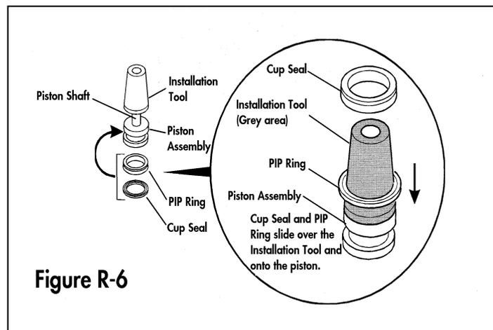
3. Lightly lubricate the cylinder in the pump body with silicon grease. Slide the finished piston assembly, shaft first, into the pump body from the side of the pump body that faces the check valve plate. Install the large o-ring (8012588) into its groove in the pump back plate and lower the pump back plate over the piston shaft. The side of the back plate with the large o-ring should be facing the pump body. See **Figure R-7**.
