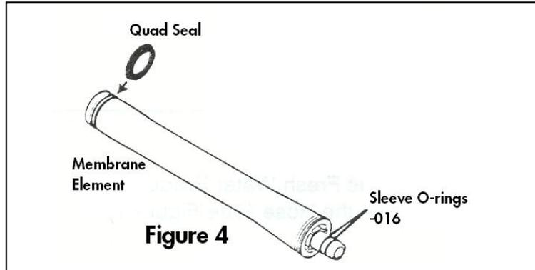
6. Install two new O-rings -016 on the male end of the Membrane (see Figure 4).
