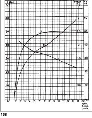
Characteristic curves for alternator type Marelli AA 125 R 14V
