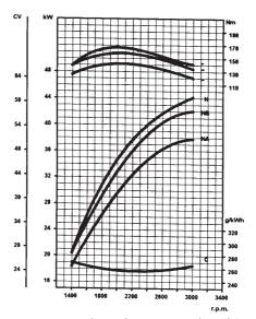
N (80/1269/CEE - ISO 1585) AUTOMOTIVE RATING: intermittent operation with variable speed and variable load.
