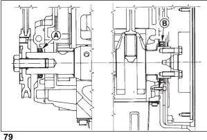
Crankshaft front and rear oil seal
