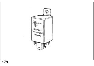
Glow plug controller relay with coolant temperature sensor
