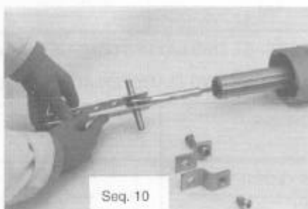
Seq. 10 Montez l'axe PROFURL. Fit the PROFURL clevis pin.
