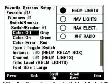
Figure 253 – Configuration of an Individual Switch/Breaker
