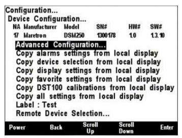
Figure 61 – DSM150/DSM250 Remote Configuration Screen
