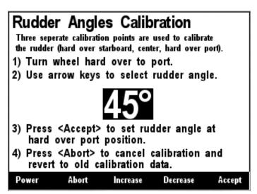
Figure 148 – RAA100 Port Rudder Angle Calibration
