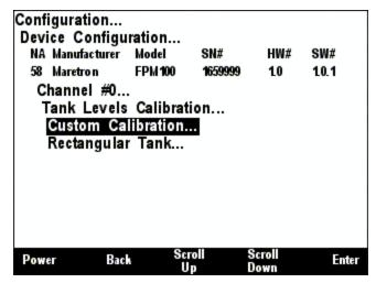
Figure 100 – FPM100 Tank Levels Calibration Menu
