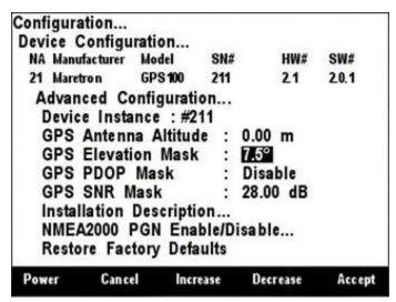
Figure 111 – Configuring Satellite Elevation Mask on a GPS100
