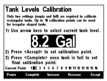
Figure 191 – Intermediate Level Calibration
