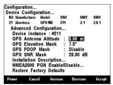
Figure 110 – Configuring Antenna Altitude on a GPS100
