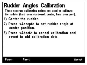
Figure 147 – RAA100 Center Rudder Angle Calibration
