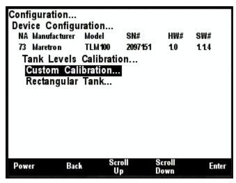
Figure 206 – Performing Custom Calibration of the Tank Level Monitor
