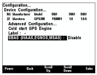
Figure 124 – Configuring SBAS on a GPS200
