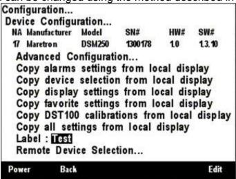
Figure 70 – DSM150 Label Configuration
