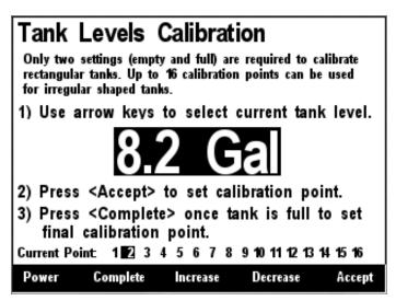
Figure 209 – Intermediate Level Calibration
