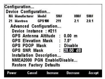
Figure 113 – Configuring SNR Mask on a GPS100
