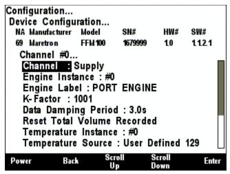
Figure 88 – FFM100 Channel #0 First Configuration Screen (Differential Mode)
