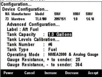
Figure 186 – Configuring the Tank Capacity
