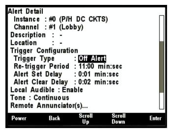
Figure 264 – Trigger Configuration – Data Unavailable Alert
