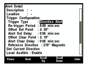
Figure 271 – Trigger Configuration – Direction Alert
