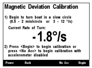
Figure 174 – SSC200 Magnetic Deviation Calibration Start Screen
