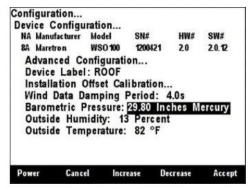
Figure 232 – Setting the Barometric Pressure
