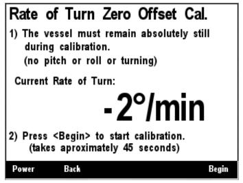
Figure 178 - SSC200 Rate of Turn Zero Offset Calibration Screen
