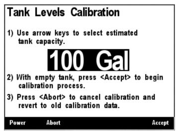
Figure 102 – Tank Levels Calibration Capacity Estimation
