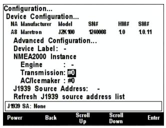
Figure 135 – J2K100 NMEA2000 Transmission Instance Configuration
