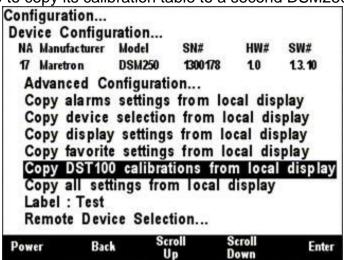
Figure 68 – DSM150/DSM250 Copy DST100 calibrations from local display
