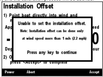
Figure 228 – WSO100 Configuration Aborted Due to Low Wind Speed
