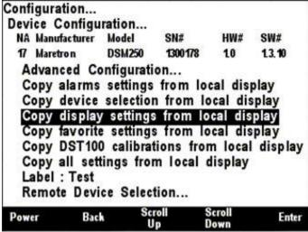
Figure 65 – DSM150/DSM250 Copy display settings from local display
