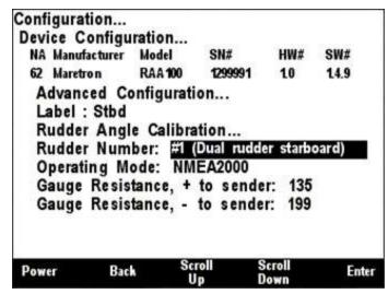
Figure 150 - RAA100: Setting the Rudder Number
