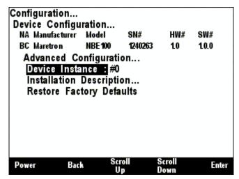
Figure 139 – NBE100 Advanced Configuration Screen
