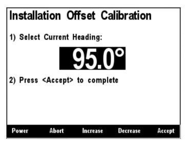
Figure 172 - SSC200 Installation Offset Calibration Screen
