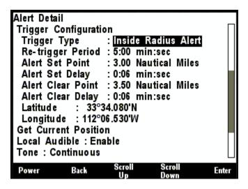
Figure 268 – Trigger Configuration – Inside Radius Alert
