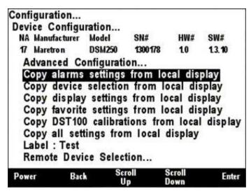
Figure 63 – DSM150/DSM250 Copy alarms settings from local display
