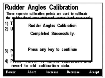
Figure 149 – RAA100 Custom Rudder Calibration Confirmation Screen
