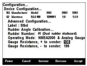
Figure 152 – RAA100: Setting the + to Sender Gauge Resistance
