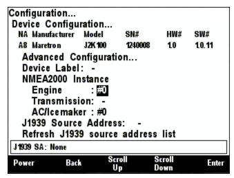
Figure 134 – J2K100 Engine Instance Configuration
