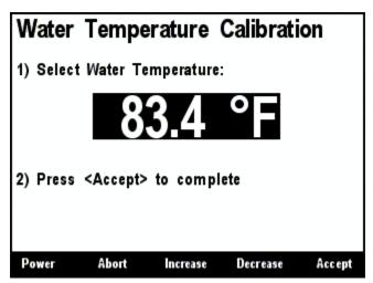
Figure 33 – Airmar Temperature Transducer Water Temperature Calibration Screen
