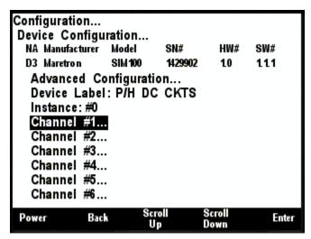
Figure 158 – SIM100 Configuration Screen
