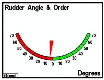
Figure 239 – Rudder Angle Gauge Display Example
