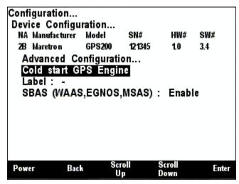
Figure 123 – Performing a Cold Start of the GPS200
