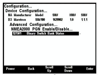
Figure 164 – SMS100 NMEA 2000® PGN Enable/Disable Screen
