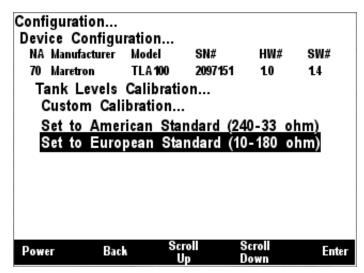
Figure 195 – European Standard Sender Calibration
