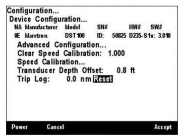
Figure 76 – Resetting the DST100 Trip Distance Log
