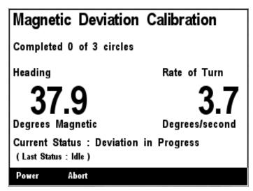
Figure 175 – SSC200 Magnetic Deviation Calibration Progress Screen
