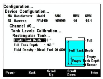
Figure 107 – Rectangular Tank Calibration
