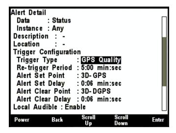
Figure 269 – Trigger Configuration – GPS Quality Alert
