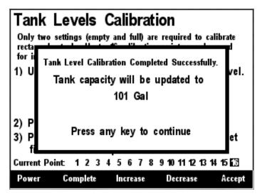
Figure 211 – Custom Tank Level Calibration Confirmation Screen
