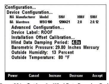
Figure 231 – Setting the Wind Data Damping Period
