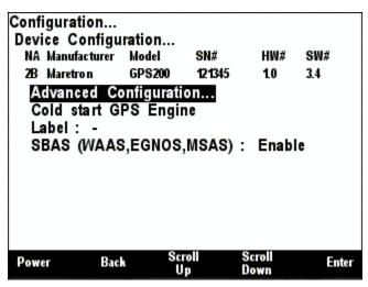
Figure 119 - GPS200 Configuration Screen
