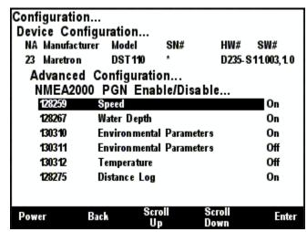
Figure 79 - DST110 NMEA 2000® PGN Enable/Disable Screen
