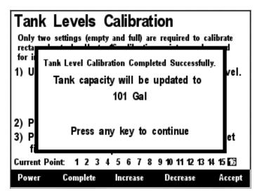
Figure 193 – Custom Tank Level Calibration Confirmation Screen
