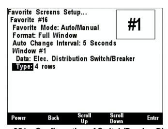
Figure 251 - Configuration of Switch/Breaker Display
