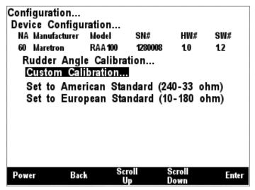
Figure 145 – RAA100 Custom Rudder Angle Calibration
