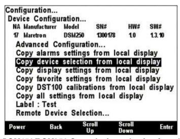
Figure 64 – DSM150/DSM250 Copy device selection from local display
