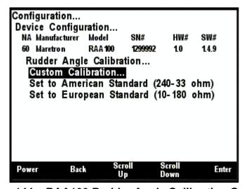
Figure 144 – RAA100 Rudder Angle Calibration Options
