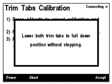
Figure 38 - EP-30 Intermediate Calibration Screen
