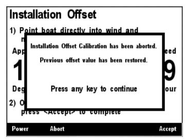
Figure 230 – Installation Offset Abort Confirmation Screen
