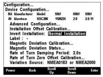
Figure 173 - Setting the Installation Orientation
