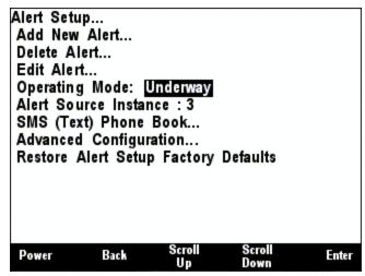
Figure 281 - Setting the Vessel Operating Mode
