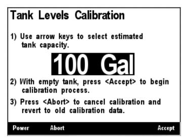
Figure 189 – Tank Levels Calibration Capacity Estimation
