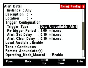
Figure 262 – Trigger Configuration – Data Unavailable Alert
