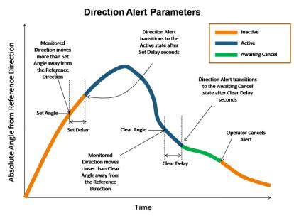
Figure 270 – Direction Alert Parameters
