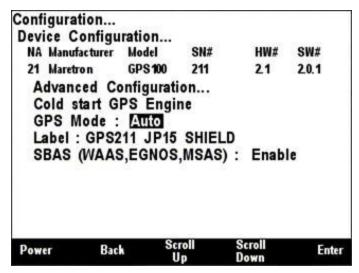
Figure 117 – Configuring GPS Operating Mode on a GPS100
