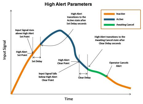
Figure 258 - High Alert Parameters
