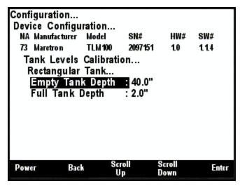
Figure 213 – Rectangular Tank Calibration
