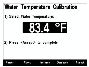
Figure 81 – DST110 Water Temperature Calibration Screen
