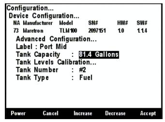
Figure 204 – Configuring the Tank Capacity
