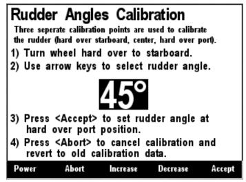
Figure 146 – RAA100 Starboard Rudder Angle Calibration
