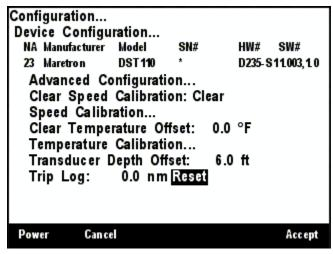
Figure 83 – Resetting the DST110 Trip Distance Log
