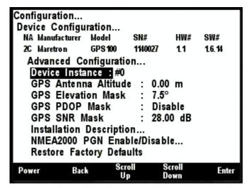
Figure 109 – GPS100 Advanced Configuration Screen
