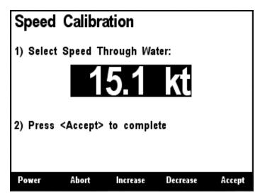
Figure 80 – Calibrating the DST110 Speed
