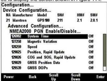
Figure 114 – GPS100 NMEA 2000® PGN Enable/Disable Screen
