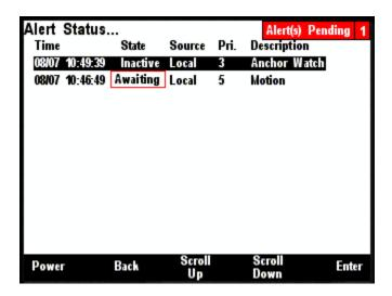
Use the **Scroll Up** and **Scroll Down** buttons to select the Alert to be accepted or cancelled, and then press the **Enter** button. An Alert Description screen will be displayed with the details of the Alert and the cursor positioned over the **Accept/Cancel Alert** entry.
