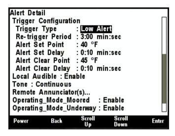
Figure 261 - Trigger Configuration - Low Alert
