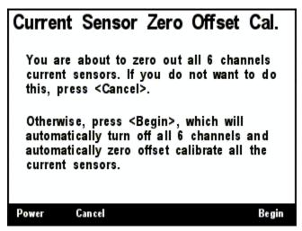
Figure 54 – DCR100 Current Sensor Zero Offset Calibration Screen
