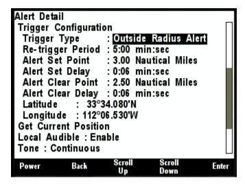
Figure 267 – Trigger Configuration – Outside Radius Alert
