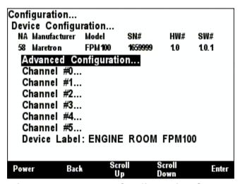
Figure 95 – FPM100 Configuration Screen
