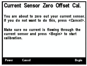
Figure 50 – Current Sensor Zero Offset Calibration Confirmation Screen
