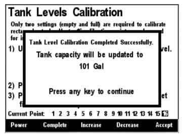
Figure 106 – Custom Tank Level Calibration Confirmation Screen
