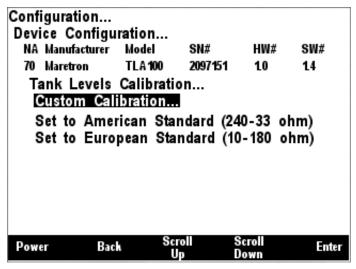
Figure 188 – Performing Custom Calibration of the Tank Level Adapter
