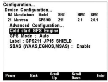
Figure 116 - Performing a Cold Start of the GPS100
