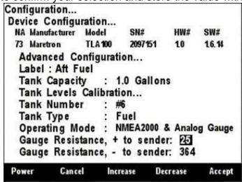
Figure 199 – Configuring the + to Sender Gauge Resistance
