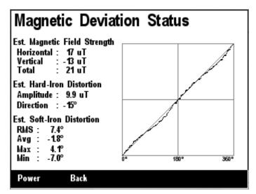
Figure 176 – SSC200 Magnetic Deviation Status Screen
