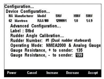
Figure 153 – RAA100: Setting the – to Sender Gauge Resistance
