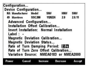
Figure 177 - Programming SSC200 Rate of Turn Damping Period
