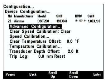
Figure 30 - Airmar Depth/Speed/Temperature Transducer Configuration Screen
