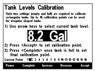
Figure 104 – Intermediate Level Calibration
