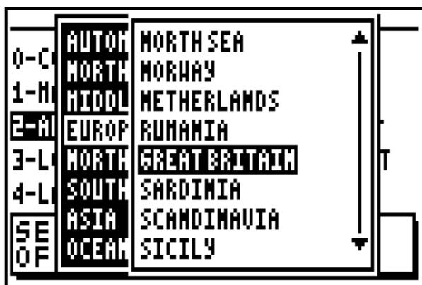
Tip: By selecting the Country of use it allows your DGPS to find its position faster than the automatic mode. When you change Country it is imperative to re-select your area of use or select the automatic mode.
