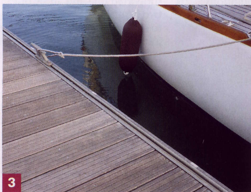
3 In slow ahead, surge the rope until the bow is in position
