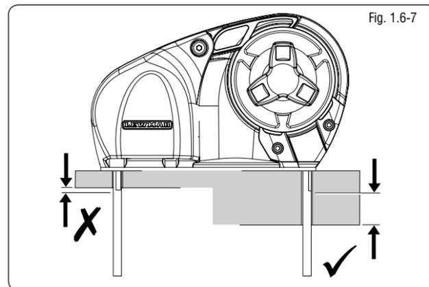
**DO NOT** use a permanent adhesive/sealant, e.g., 5200 to the base of the windlass, any mounting pad or around the studs.
