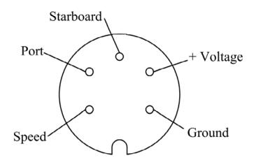
Masthead transducer connector
