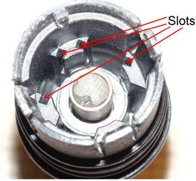
Module Housing showing the slots for the magnetic pickups.
