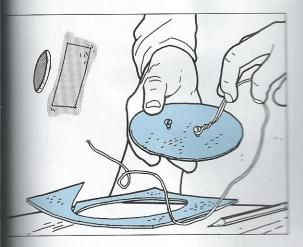
Using epoxy resin and two layers of 10-ounce cloth, lay up a backer piece on a waxed and release-coated section of the hull near the damage.
