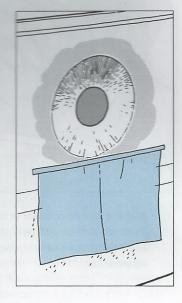
wax and releasemat a scrape of smooth plastic laminate or thin acrylic and brace it tightly mainst the hole inside. If the is flat or curving monly one direction the damage area, me backer will mume the correct turve. If the hull is mherical, lay up a water using an accent section of me bull as the mold.
