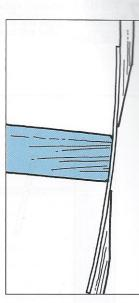
4 If you are using epoxy resin for the repair, cut all your repair pieces from 10-ounce cloth. Mix a batch of epoxy and wet out the first layer of cloth. Use a squeegee to smooth the cloth into position and to
