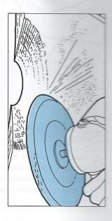
Wax the exterior surface of the skin around the hole, taking care not to get any wax on the bevel. Mask the area below the hole.
