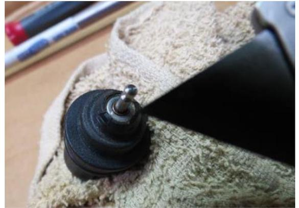
Next, using the needle-nose pliers, grasp the plastic barrel that holds the four small magnets on the inside of the housing. Pull straight out. This is a press-fit on the shaft, no glue.
