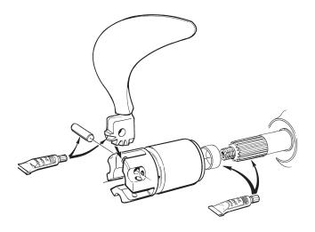
The propeller must be cleaned and lubricated once a year. Remove the propeller and clean all components thoroughly. Apply waterproof grease to the propeller blade teeth and bearing surfaces so that the propeller folds easily. Also apply waterproof grease to the studs, spacing sleeve (drive), propeller shaft and hub.
