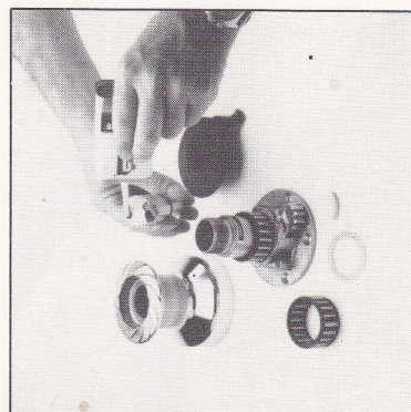
Clean spindle, grease lightly and oil pawls.
