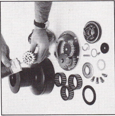
Remove spindle, lightly oil pawls and grease gear.
