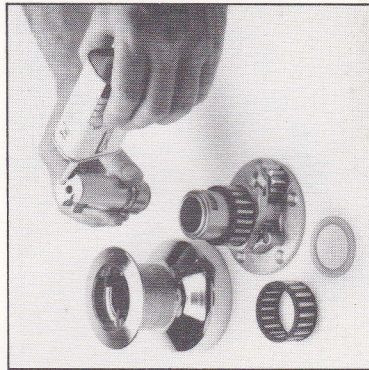
Clean spindle, grease lightly and oil pawls.
