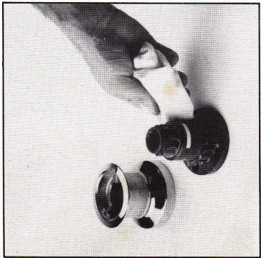
Wash centre stem and drum base with kerosene (paraffin). Dry with a non-fluffy cloth.
