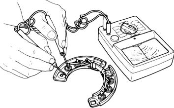
CAUTION: If a high voltage megger is used, a high voltage will be applied to the diode and the diode will be destroyed. Therefore, never test the diodes with a high voltage megger, etc.
