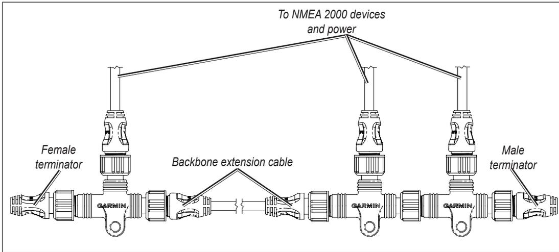
**CORRECT Linear Backbone Construction**
