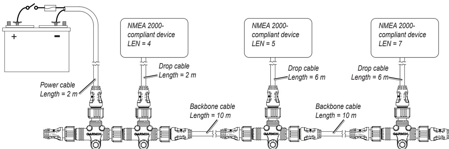
When the voltage-drop formula is applied to this example, we see that the voltage drop is less than 3.0 Vdc, so this NMEA 2000 network will function correctly when powered at the end.
