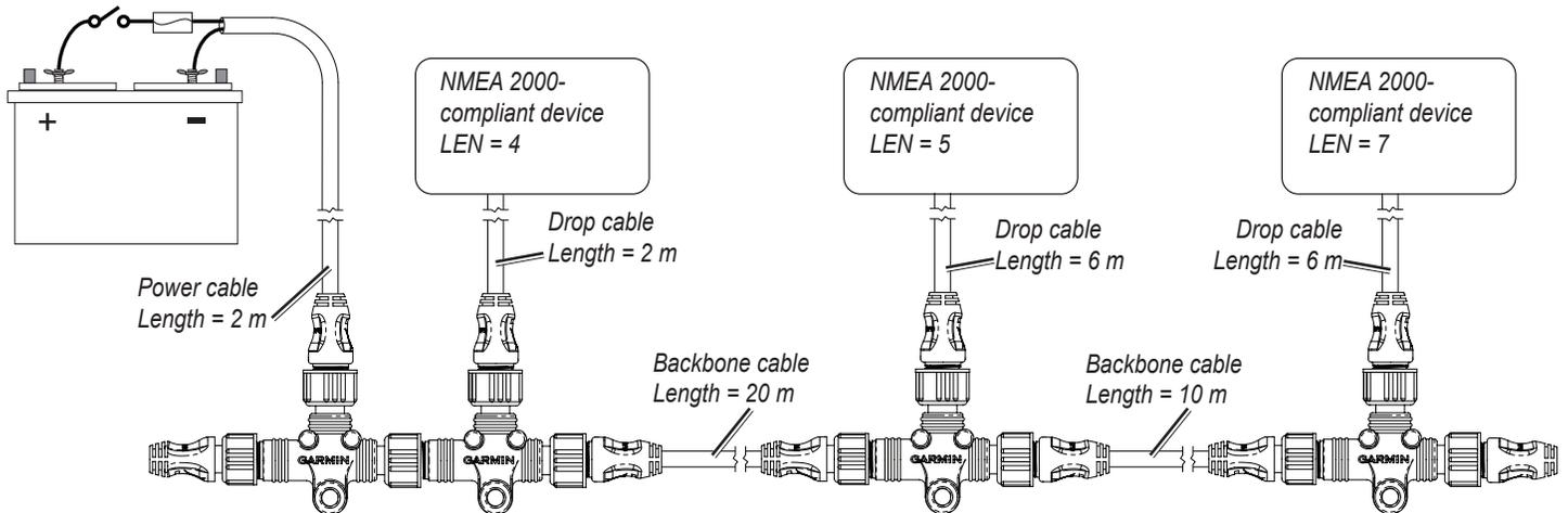
When the voltage drop formula is applied to this example, we see that the voltage drop is greater than 3.0 Vdc, so this NMEA 2000 network will not function correctly when powered at the end.
