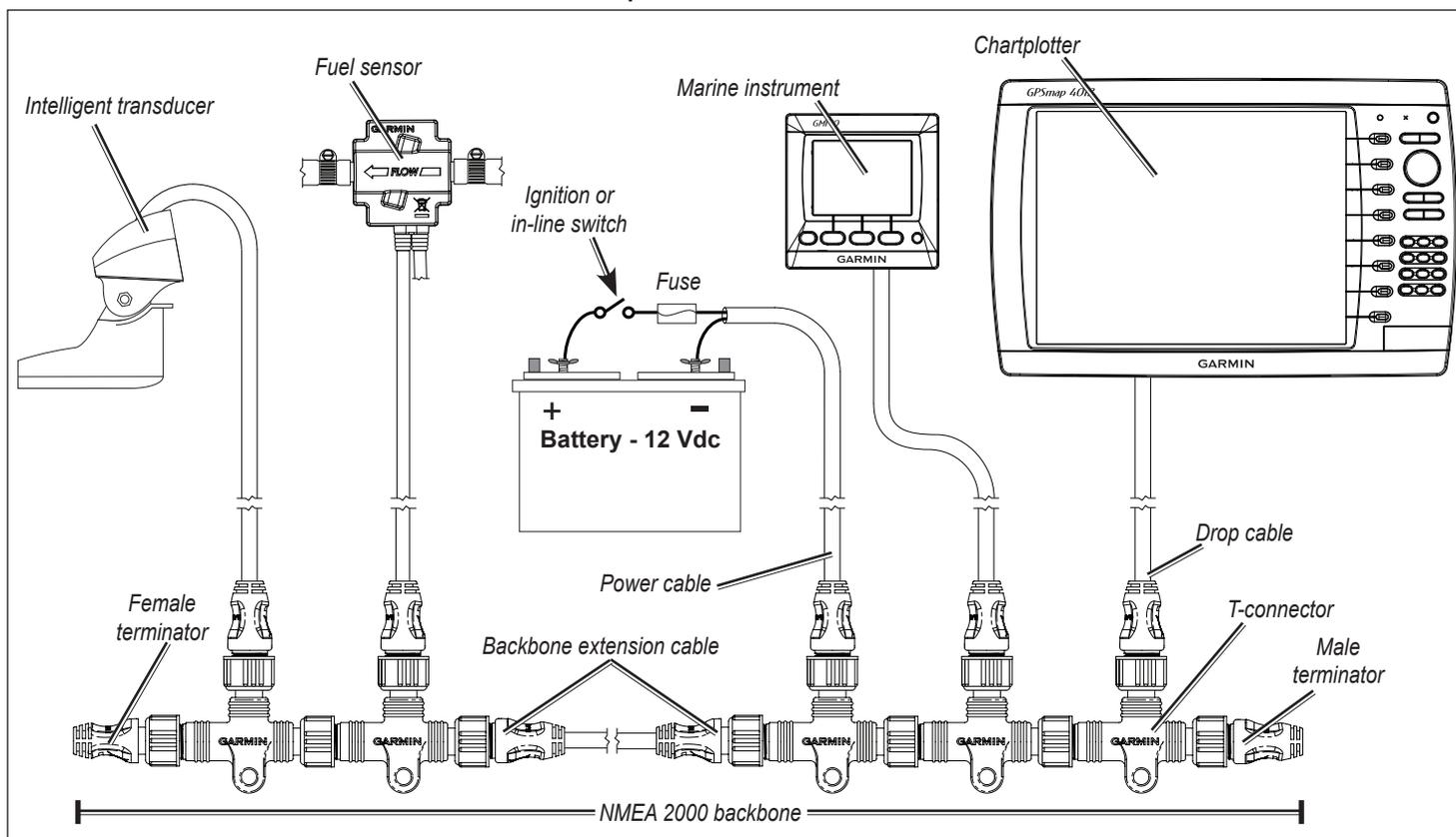
**NOTE:** This diagram illustrates the NMEA 2000 data connections to each device or sensor. Some devices or sensors can be powered by the NMEA 2000 network; others may require a separate power connection. Consult the installation instructions for each device you connect to your NMEA 2000 network to be sure you supply power to the device appropriately.
