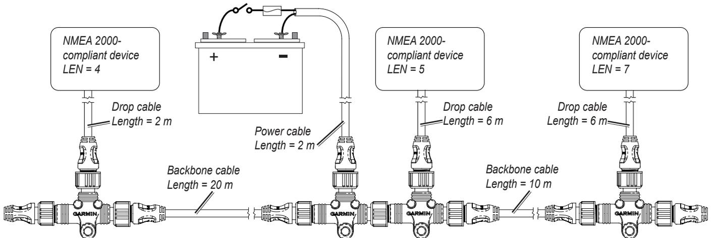
When the NMEA 2000 network is redesigned with the power source in the center, you calculate the voltage drop in both directions. If the T-connector to which you connect the power source is connected directly to another T-connector (as shown in this example), use the LEN from that device as part of the calculation for both directions.
