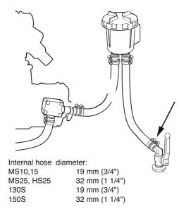
Always install a shut-off valve on the water intake. Two hose clamps for each connection should be used.
