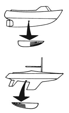
If a scoop pickup is used on a sailing boat the water intake should be facing backwards to avoid water to be pushed into the exhaust system during sailing.
