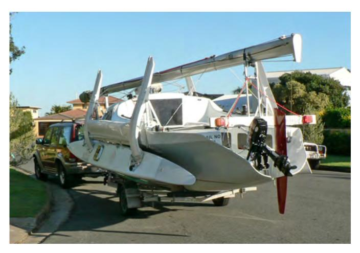
An F-22 on the trailer, with outboard and daggerboard rudder. This type of rudder can be lifted fully up for local trailering or removed altogether for long distance trips. Note separate light bar high up and well clear of water
