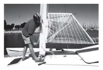
F-28 Mainsail being roller furled. Note foot being used to control halyard.
