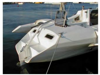
F-33 daggerboard rudder, with blade fully down
