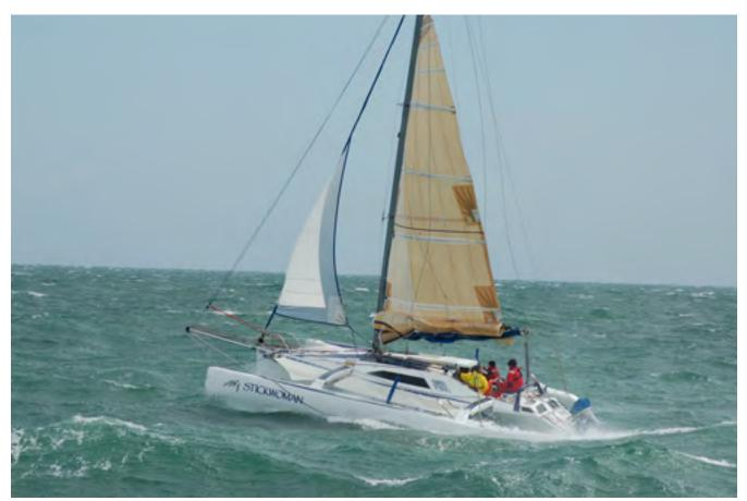
Set up and sailed properly, a Farrier design is a very safe, yet very fast boat. This F-9AX is handling some very rough conditions in South Australia quite comfortably, by being well reefed
