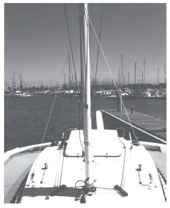
Mast raising wires may need to stay attached until <u>after</u> the boat is unfolded, depending on model. F-28 shown.
