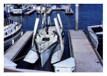
position, or lowering the mast in extreme conditions. Folded stability without the mast is very good, and the folded boat can actually self right up to even a 80 to 85 heel angle - but don't risk it.
