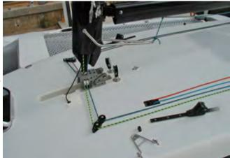
F-33 Mast Rotator Arm & attached to boom for self tacking
