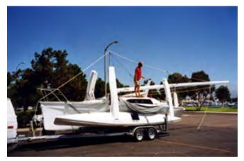
Mast raising pole in position on an F-28 with winch line connected to jib halyard, ready to raise mast. Depending on design, take care that rotating mast is restrained once up so that it cannot topple forwards. This can be done by using the Corsair type Highfield Lever to connect shrouds to float
