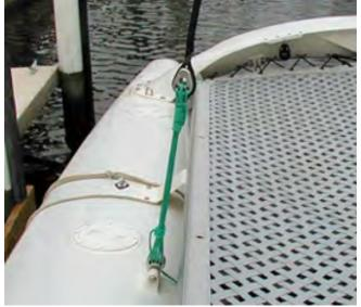
Turnbuckles have now been replaced by deadeyes and lashing on later models - much lighter and easier on boat
