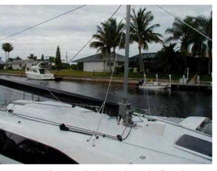
Raising wire Deck Loops - these work well to anchor raising wires as they can fold down to be flush on deck when not in use. F-33 mast step with raising pole yoke shown above and below left. The same basic mast raising setup applies for
