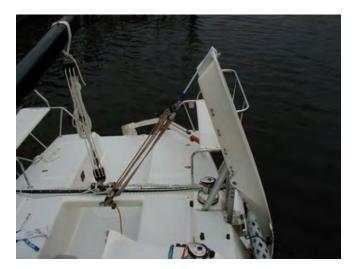
very light boat, as the boat will have heeled towards the extended float, meaning the folded float will have to be moved upwards when initially folding. This will improve for most as the boat is loaded with cruising gear, but racers kept light will continue to see this problem
