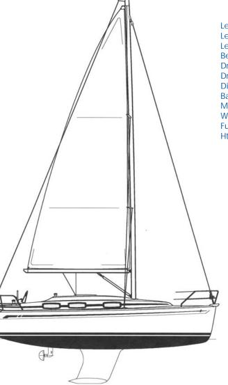
Length overall 31' Length hull 30' Length waterline 27'1" 10'9" Beam Draft standard 4'7" Draft (deep option) 6'1" Displacement 9,240 lbs. Ballast 2,200 lbs. Mainsail & genoa 555 sq. ft. (appx.) Water tank 40 gal. (appx.) Fuel tank 25 gal. (appx.) 46'3" Ht. of mast above waterline
