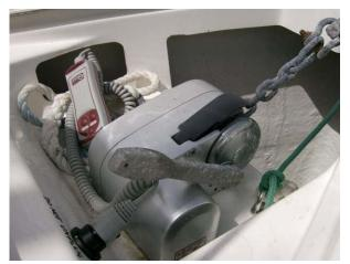
If you lose power to your windlass, start the engine and give it some revs, to make sure you have not just got a low battery voltage. Then make sure the windlass breaker with the anchor icon is in the 'on' position on the 12 volt panel. If there is still no power, check the location of the windlass fuse and make sure this has not tripped out. If you still have no power, you can operate the windlass manually.
