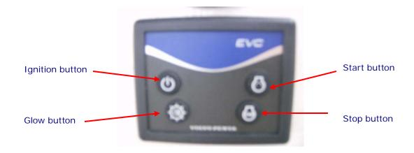
Should you hear an engine alarm during operation, check which light is on and immediately shut down the engine-CALL HORIZON
