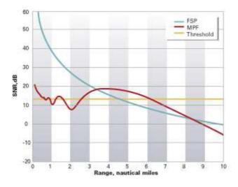
FSP Free space propagation: Propagation in vacuum with no physical objects that disrupt or distort the radiated beam
