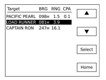
Each target shown in the target list indicates the CPA as well as the bearing and range from your vessel to the target. This facilitates visual identification. In setup mode you can change whether bearings are shown as true, magnetic, or relative to your vessel's heading.
