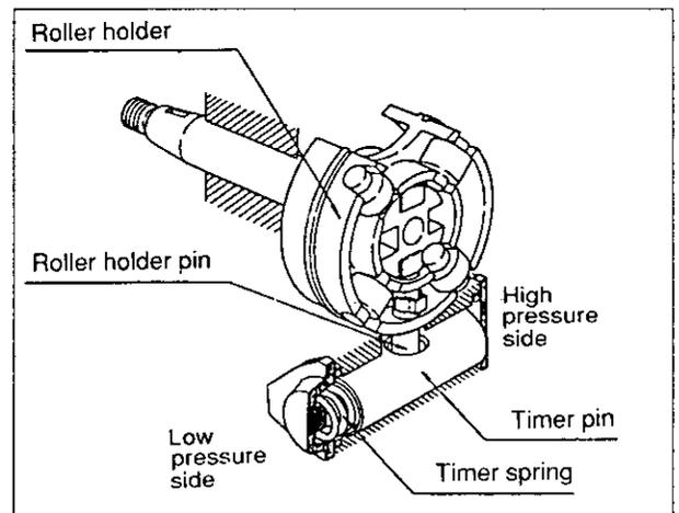
When the piston moves in the direction where the timer spring is shrunk, a lead of angle takes place (the roller holder moves in the reverse direction of rotation) to advance the injection timing. That is, the timer controls the injection timing according to the fuel oil pressure in the pump house.
