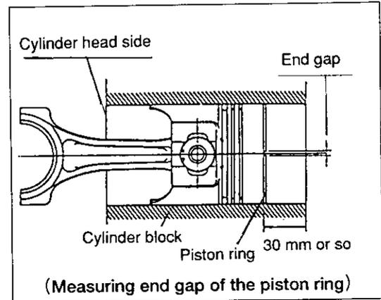
③ Replacing the piston ring
