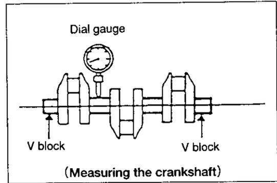
③ Measuring crank pin and crank journal
