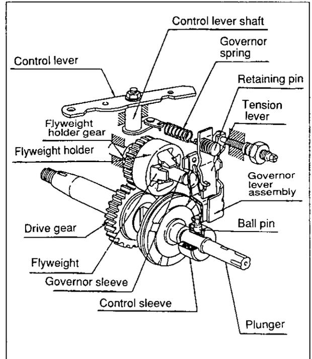
②The governor spring located at the top of it is connected to the tension lever with the retaining pin and the governor spring end face is connected to the control lever through the control lever shaft.
