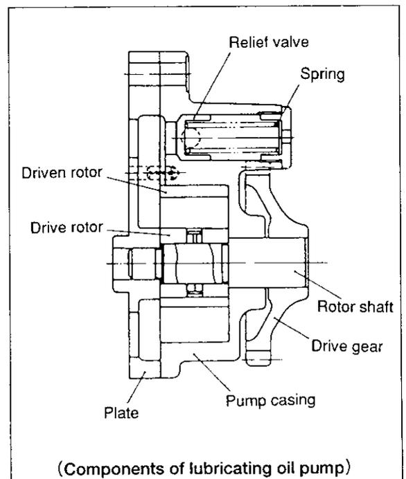
② Disassembling the lubricating oil pump
