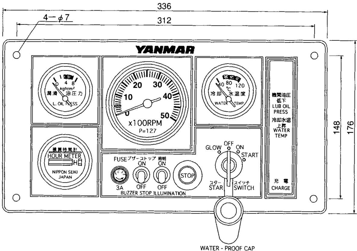
**YANMAR MARINE DIESEL ENGINE
