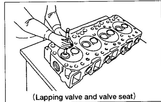
⑤ Replacing the valve seat
