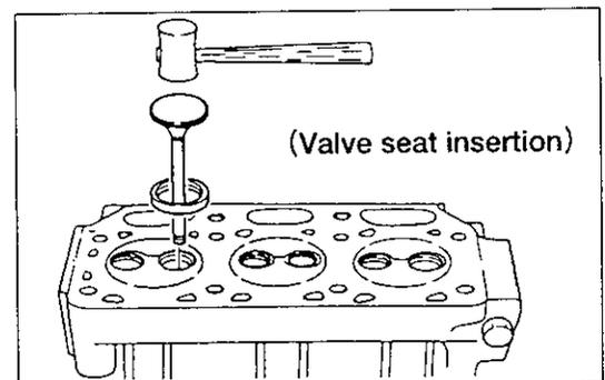
(3) Intake/exhaust valve and valve guide
