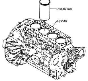
NOTE: If it is difficult to pull out the liner, tap the bottom of the liner with a plastic hammer.
