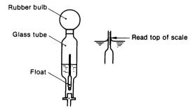
The battery is fully charged if the specific gravity is 1.260 at an electrolyte temperature of 20°C. The battery is discharged if the specific gravity is 1.200 **-**4JH Series
