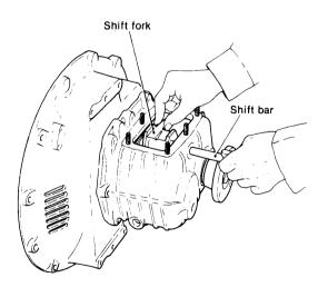
(1) Put the shift fork into neutral before installing.
