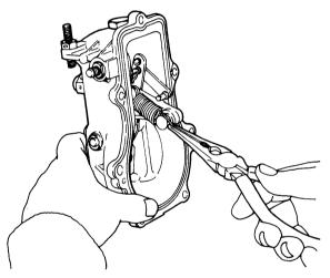
(11) Pull the governor link as far as possible towards the governor case mounting surface, insert the governor link pin in the fuel control rack pin hole and fit the snap pin on it.
