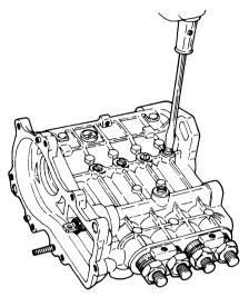
(10) Use a hammer handle or the like to push up the roller guide from the bottom of the pump, and remove the plunger spring support plate.
