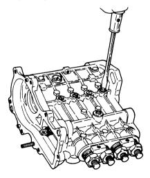
(12) Fit the bearings to both ends of the camshaft, and insert from drive side by lightly tapping.
