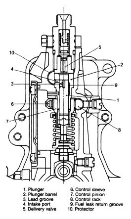
The fuel injection pump supplies pressurized fuel to the injection nozzles through the action of the plunger. The plunger reciprocates in the plunger barrel through a fixed stroke and is lapped for a precise fit. A lead groove is helically cut in the plunger, and this leads to a connecting groove which goes to the top of the plunger.
