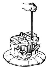
2) Remove the clutch case cover from the clutch case.
