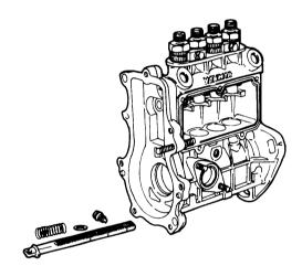
(16) Loosen the delivery valve retainer stop bolt, and remove the delivery valve holder stop.
