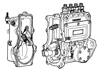
(6) Remove the stop lever return spring from the governor lever shaft.
