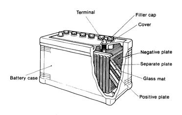
The battery utilizes chemical action to convert chemical energy to electrical energy. This engine uses a fead acid battery which stores a fixed amount of power that can be used when required. After use, the battery can be recharged and used again.
