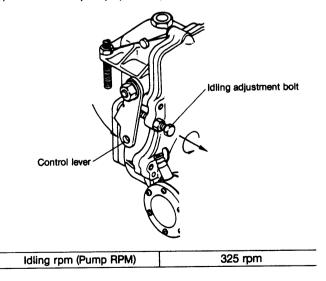
(2) Measure the injection volume while lowering the governor control lever to the idling position, and adjust the position of the control lever with the idling adjustment bolt to bring it to specified value.
