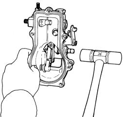
NOTE: After mounting the governor lever assembly, make sure the governor lever assembly moves smoothly.
