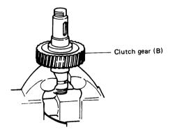
NOTE: Check that the clutch gear (B) rotates smoothly.
