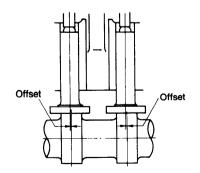
NOTE: When removing tappets, be sure to keep them separate for each cylinder and intake/exhaust valve.
