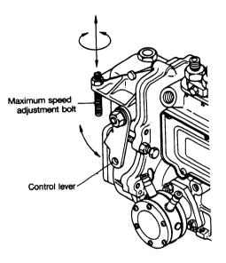
(2) Check maximum RPM at no load
