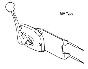
The MV type controller has been designed so that operation of the clutch and throttle can be effected with one lever. When the button next to the control lever is pulled out with the lever in the central position, it holds the clutch in the neutral position so that the throttle can be opened all the way and warm up the engine.
