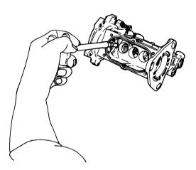
Plunger inserting tool
