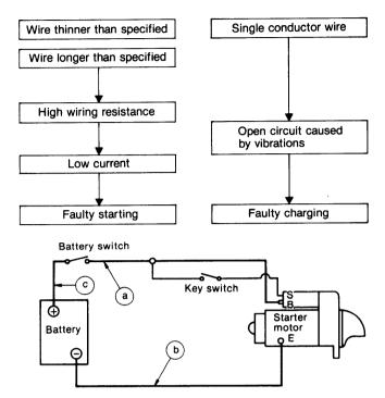
The overall lengths of the wire between the battery (+) terminal and the starter (B) terminal, and between the battery (-) terminal and the starter (E) terminal, should be determined according to the following table.
