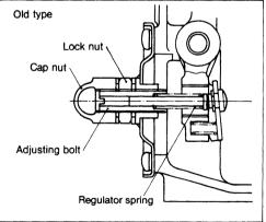
This governor is all-speed, directly connected to the YPES-CL fuel injection pump. The construction will be explained with the cutaway views.
