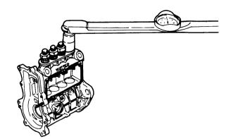
(18) Remove the delivery valve assembly.
