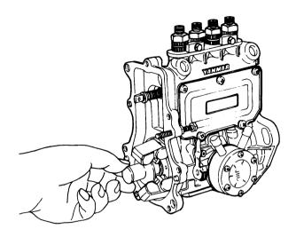
(15) Turn the governor weight with a box spanner two or three times to loosen it, stopping it with the hole in the fuel coupling ring or holding the coupling with a vise.
