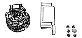
(5) Disconnect the soldered joint of the stator lead wire, and remove the diode and brush regulator assemblies from the stator at the same time.
