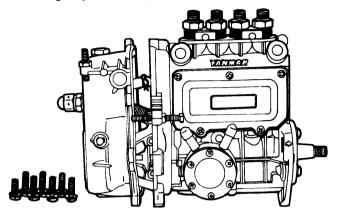
(4) Pull out the governor link snap pin by inserting needle nosed pliers between the fuel pump and governor case. case.
