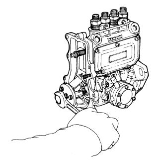
(2) Remove the fuel feed pump.
