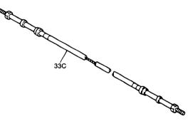
Use only Super-Responsive Morse Control Cables. These are designed specifically for use with Morse control heads. This engineered system of Morse cables, control head and engine connection kits ensures dependable, smooth operation with an absolute minimum of backlash.
