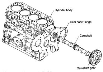
(3) Measure the camshaft side gap.
