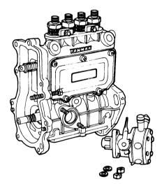
(3) Remove the fuel pump side cover.
