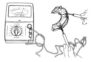
CAUTION: Do not use high tensile insulation resistance such as meggers, etc. for testing. The diode may burn out.
