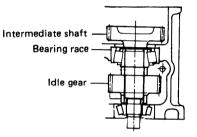
(3) Drive the outer bearing race into the clutch case.
