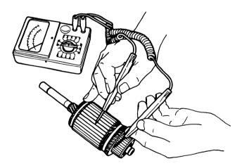
Checking armature windings for insulation faults.
