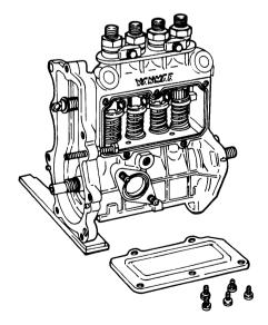
(4) Turn the camshaft until the roller guide is at the maximum head, and insert the plunger spring support plate in between the plunger spring washer B (lower side) and fuel pump unit.
