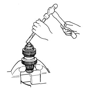
NOTE: Use the clutch gear (A) side nut which is used before dismounting for the clutch gear (B) end nut. This not to make the calked portion to the same point.
