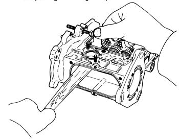
NOTE: 1. Face the roller guide stop groove up, and align with stop screw hole on pump.
