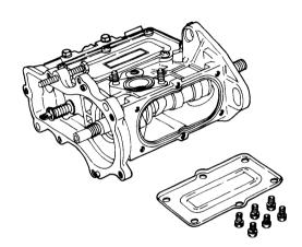
(1) Loosen the nut with a box spanner and take it off, holding it with the hole in the fuel coupling ring or holding the coupling with a vise and take out the governor weight assembly.
