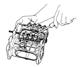
NOTE: 1. Check to make sure the match marks on the pinion/sleeve are correct before loosening the small screw on the control pinion, as the pinion and sleeve come apart when the screw is loosened. If the mark is hard to read or off center, lightly inscribe a new mark. This will serve as a guide when adjusting injection volume later.
