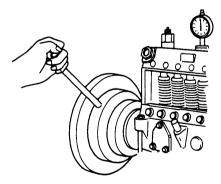
(3) Turn the camshaft, and bring cam to top dead point while watching gauge needle.
