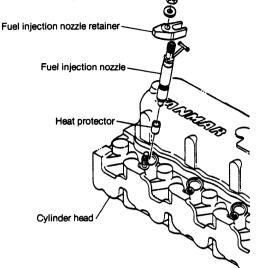
(2) Tighten the fuel injection nozzle retainer nut to the specified torque. kg-m (ft-lb)
