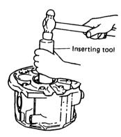
(2)Insert the clutch shaft shim, Lube oil filter case and filter into the clutch case.
