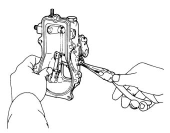
(10) Hook the governor spring on the control lever shaft and tension lever hook with radio pliers.
