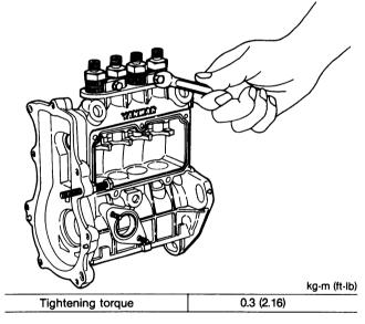
NOTE: Overtightening can upset the delivery retainer and cause oil leakage.
