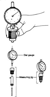
(2) Remove the injection pump delivery retainer, take out the delivery valve assembly, insert the top clearance gauge and tighten by hand.
