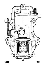
(9) Put a rod 8mm (0.3150in.) in dia. or less in one end of the governor lever shaft, and tap the governor shaft until the O-ring comes out the other side of the governor case.
