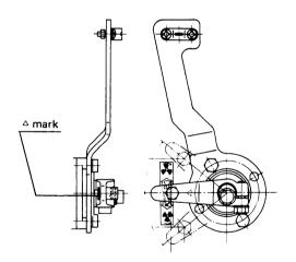
(4)Insert the shifter spring and shifter to the shift lever shaft
