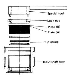
Chapter 7 Reduction and Reversing Gear 5. Disassembly
