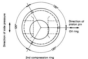
(5) The oil ring is provided with a coil expander. The coil expander joint should be opposite (staggered 180°) the oil ring gap.
