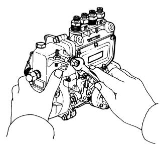
NOTE: Move the control lever back and forth to make sure that the entire link moves smoothly.
