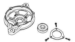
(4) Remove the nut, the brush-holder, and diode fixing nut at the BAT, and the terminal screws of the rear cover. Separate the rear cover from the stator (with the diode and brush holder).
