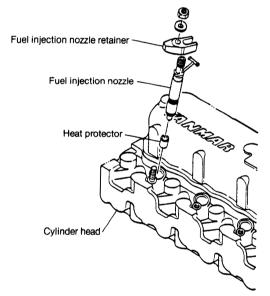
NOTE: If the heat protector stays in the cylinder head, make a note of the cylinder no. and be sure to remove it when you disassemble the cylinder head.
