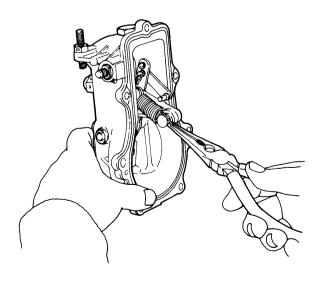
Printed in Japan 0000A0A1647 (8) Remove the snap-rings on both ends of the governor lever shaft.
