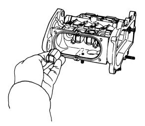
NOTE: When you stand the fuel pump up, all of the roller guides drop out at one time. Therefore, first remove the stop bolt for one cylinder at a time, and then the roller guide for each cylinder—continue this process.
