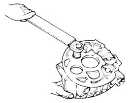
NOTE: Thread of the locknut is left-handed.
