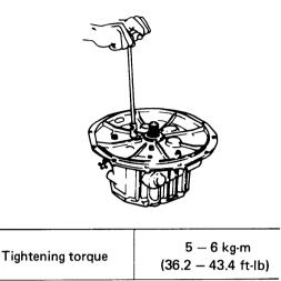
NOTE: Apply non-drying liquid packing to the maching surface of the mounting flange and the clutch case.
