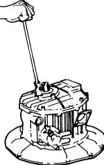
(6) Insert the oil seal, output shaft coupling, O-ring and the end nut into the output shaft.
