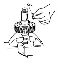
(6)Drive in the driving gear and inner bearing race using the inserting tool.
