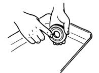
(3)Lap the clutch gear's cave and drive cone, pushing them together by hand
