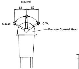
The stroke between the neutral position  $\rightarrow$  C.W. position (S2), and the neutral position  $\rightarrow$  C.C.W. position (S1) must be equalized.
