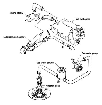
Printed in Japan 0000A0A1647 Fresh water line [ENGINE MODEL: 4JH-HTE & 4JH-DTE] S changer /Filler cap (with pressure control valve)
