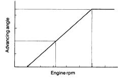
The advancing characteristics can be changed by changing the profile of the side of the weight and the spring constant of the spring.
