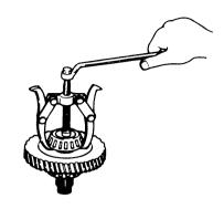
(2) Fix the input shaft gear in a vice, and remove the lock nut with a special tool.
