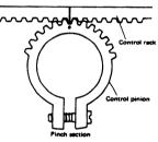
(6) While holding the pinion with one hand and keeping it aligned with the match mark, fit in the sleeve, and lightly tighten the small pinion screw.
