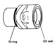
(2) Insert the shift lever shaft to the side cover
