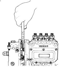
(5) The governor and fuel pump come apart by sliding the governor case and fuel pump apart and pulling out the link pin of the fuel control rack.
