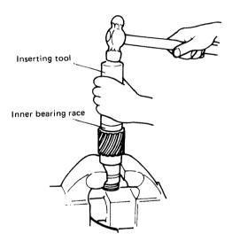
(3) Assemble the needle bearing and clutch gear (B)
