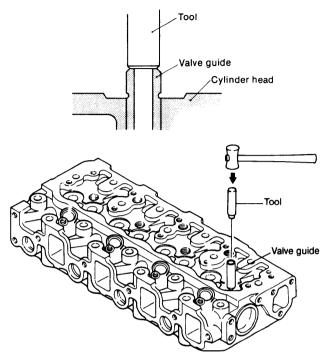
The intake valve guide and exhaust valve guide are of different shapes/dimensions. The one with a groove around it is the exhaust valve guide and the one without is the intake valve guide.
