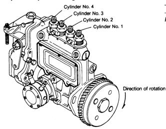
(1) Set the governor control lever to the operating position and fix (bring plunger to the effective injection range), turn the camshaft clockwise, and check the injection starting time (FID) of cylinder No.1 (start of discharge of fuel from the delivery retainer).
