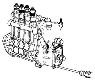
(14) Insert the control lever in the control lever shaft, and tighten the nut.
