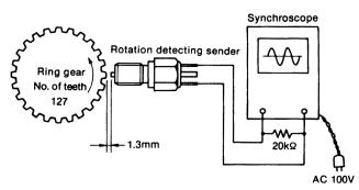
\* Check the output wave pattern and number of pulses when carrying out the output voltage measurement.
