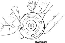
Printed in Japan 0000A0A1647 (4) Valve contact/mounting
