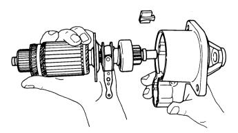
(2) Remove the pinion stopper clip.
