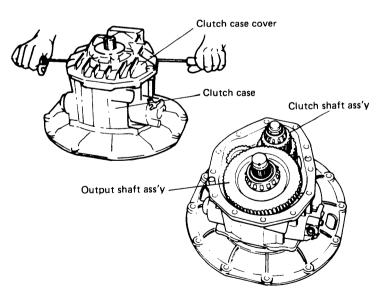
NOTE: To remove the case cover and the case, insert two drivers into the two depressed points at the joint between the case cover and the case. This makes removal easy. (9) Removing the output shaft assembly and clutch shaft assembly.
