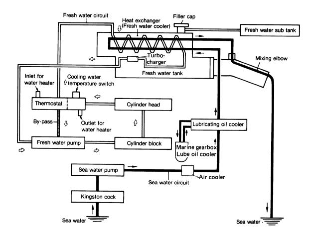
NOTE: Air cooler, marine gear box, lube oil cooler, and water-cooled turbocharger are only for models 4JH-HTE and 4JH-DTE.
