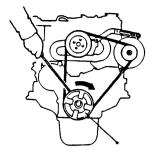
(3) If injection timing is off, change the mounting position using the long hole in the injection pump mounting flange. Turning the fuel feed pump towards the cylinder block slows timing down, while movement in the other directon makes it faster.
