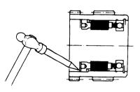
(10)Insert the input shaft into the input gear assembly.(11)Drive in the inner bearing race onto the input shaft end.
