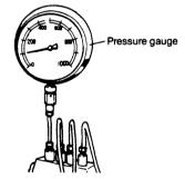
(2) After pressure rises to the above value, measure the time it takes to drop from  $100 \sim 90 \text{ kg/cm}^2$  (1422  $\sim 2702 \text{ lb/in.}^2$ ).
