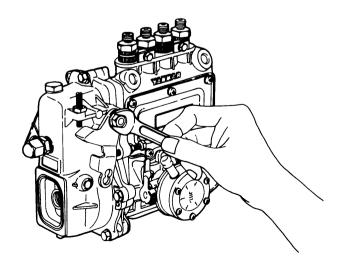
(3) Remove the governor case bolt. Remove the governor case (parallel pin) from the fuel pump unit while lightly tapping the governor case with a wood hammer. Create a gap between the governor case and fuel pump by moving only the moving parts of the governor lever.
