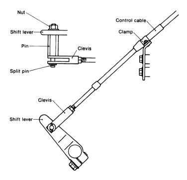
When the cable is attached to the hole 52mm (2.0472in.) from the center of the rotation of the shift lever, these strokes must be 30mm (1.1811in.)
