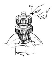
(5) Fit the cup spring, spring retainer and thrust collar (A) and drive in the inner bearing race using the inserting tool.
