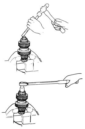
NOTE: Remember that the nut has a left-handed thread.
