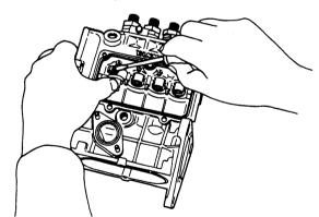
NOTE: Fitting of sleeve; Face towards small pinion screws and align with match mark.
