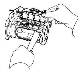
NOTE: The plunger spring may make the roller guide and plunger, etc. fly out when the plunger support plate is removed.
