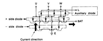
U.V.W.: terminal from the stator coil
