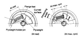
The spring is pressed against the center of the flyweight. As rpm increases, the centrifugal force of the two flyweights increases, compresses the timer spring, and the position of the weight holder and flange changes due to the movement of the curved surface of the weight, changing the injection timing. Accordingly, as the spring is compressed (according to the rise in rpm advancing the timing), the advancing angle remains proportional to rpm.
