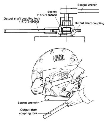
(3) Remove the output coupling with O-ring.
