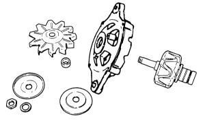
(3) Remove the Ø5mm (Ø0.1969in.) screw from the front cover, and then remove the ball bearing.
