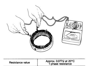
2) Stator coil insulation test
