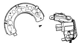
2) To replace the IC regulator, disconnect the soldered joint of the IC regulator and pull out the two bolts. Do not remove these two bolts except when replacing the IC regulator.
