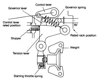
(4) No load max. rpm control
