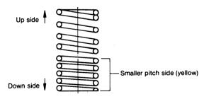
NOTE: The pitch of the valve spring is not even. The side with the smaller pitch (yellow) should face down (cylinder head) when assembled.
