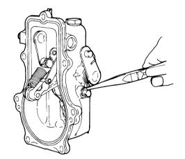
(7) Use needle nose pliers to unhook the governor spring from the tension lever and control lever shaft.
