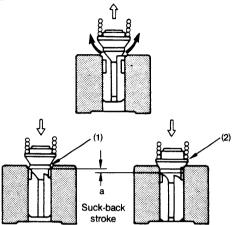
At this time, the suck-back collar (1) blocks off the fuel injection pipe and the delivery chamber, and the valve continues to descend until the seat (2) comes in contact with the barrel. The fuel oil pressure in the fuel injection pipe decreases proportionately with the lowering of the valve (due to increased volume).
