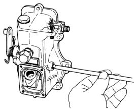
(10) After you remove the O-ring, lightly tap the end of the shaft that you removed the O-ring from, and remove the governor lever shaft. Then remove the governor shaft assembly and washer.
