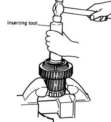
(3) Assemble the needle bearing and clutch gear (A)
