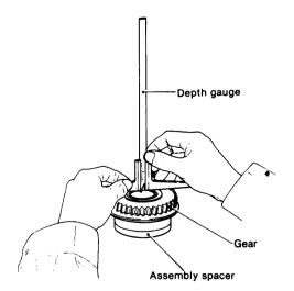
NOTE: As mentioned in section 5-3. (5), if no parts need to be replaced, the adjusting plate can be reused without adjustment. 1) Position the assembled large gear on the assembly tool so that the spline part is on the bottom; insert the spacer and bearing inner race into the gear.
