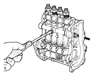
NOTE: Be careful not to lose the spring or rest on the control rack.
