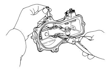
(8) After you have mounted the O-ring, tape the governor lever in the opposite direction, and mount the E-shaped stop rings on the grooves at both ends.
