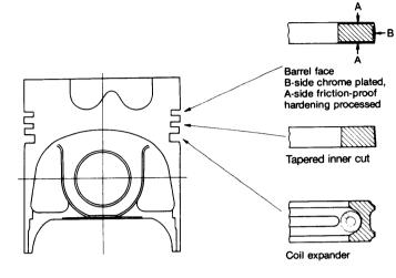
Measure the thickness and width of the rings, and the ring-to-groove clearance after installation. Replace if wear
