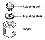
(Greater shim thickness decreases top clearance and smaller shim thickness increases top clearance).
