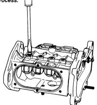
(12) Remove the plunger, plunger spring and lower washer from the lower part of the pump.
