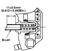
Mount the insulation tube on the terminal surface.
