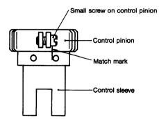
2. Keep parts separate for each cylinder.(14) Remove the control pinion, sleeve and upper rest.
