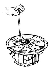
(11)Removing the input shaft assembly. Draw out from the mounting flange side of the case.
