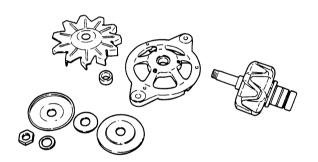
(3) Remove the Ø5mm (Ø0.1969in.) screw from the front cover, and then remove the ball bearing.
