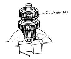
NOTE: Check that the clutch gear (A) rotates smoothly.
