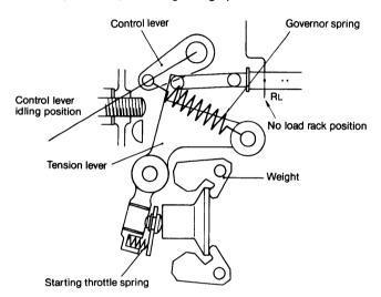
(3) Rated load max. rpm control
