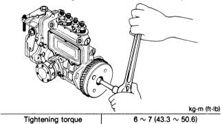
NOTE: The box nut is tightened by turning it right looking from the drive side.
