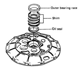
(3) Fit the mounting flange onto the clutch case, and tighten the bolt.
