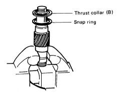
(2)Drive in the inner needle bearing race using the inserting tool.
