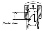
This setting is normally used for starting and max. output operation.
