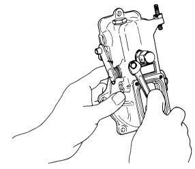
(13) When you need to pull out the control lever shaft, tap the end of the shaft with a wood hammer.
