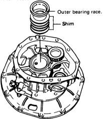
(2)Drive the shims and the outer bearing races into the clutch case cover
