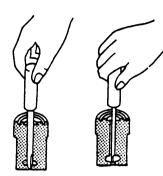
(5) Clean off the carbon on the tip of nozzle with a piece of wood.
