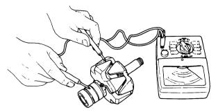
4) Check the rear side ball bearing. If the rotation of the bearing is heavy, or produces abnormal sounds, replace the ball bearing.
