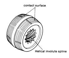
(2)Check the helical involute spline for any abnormal condition on the tooth surface, and repair or replace the part should any defect be found. (3)Measure the amount of wear on the tapered contact surface of the drive cone, and replace the cone when the wear exceeds the specified limit.
