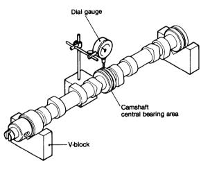
NOTE: The reading on the dial gauge is divided by two to obtain the extent of bending.
