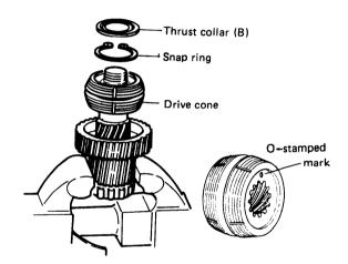
NOTE: Insert it keeping the O-stamped make surface toward the clutch gear (B) side.
