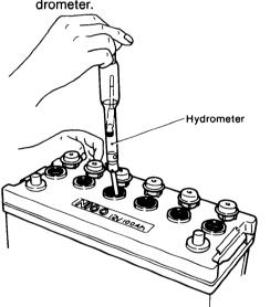
Take the specific gravity reading at the top of the scale of the hydrometer.
