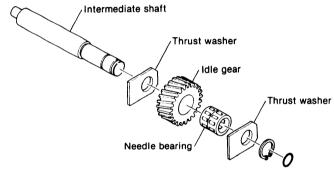
Needle bearing dimensions, staining. Check the surface of the roller to see whether the needle bearing sticks or is damaged. Replace if necessary.
