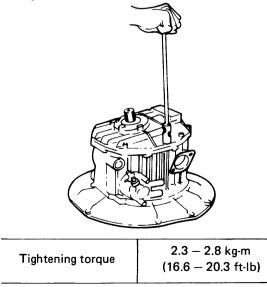
(5)Insert the outer bearing race, shim and the output shaft cover, and tighten the bolt.
