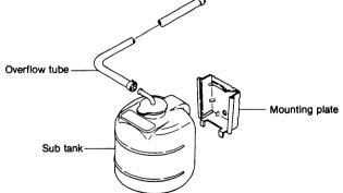
NOTE: Make sure that the overflow pipe of the sub tank is not submerged in bilge. If the overflow pipe is submerged in bilge, water in the bilge will be siphoned into the fresh water tank when the water is being cooled.
