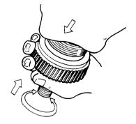
(5)After lapping them, wash them with washing oil. The lapped parts should be cleaned completely.
