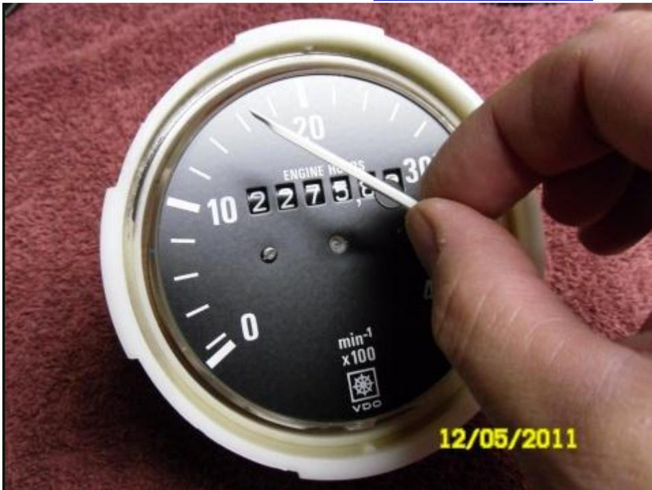
{ODG: take a picture or make a mark to where the needle points before removing. There is an internal stop with this style Tachometer/hour meter: no needle rest. Gently hold the center of the needle and gently rotate counter-clockwise. You may have to make several revolutions and the needle will start to feel loose. Gently use your first finger and thumb to pluck the needle off. The small shaft that the needle is pressed onto can be damaged if you try to just pull the needle straight off. }
