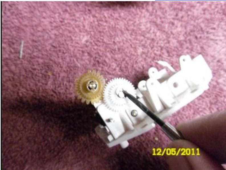
*{ODG: Remove the c-clip that secures this gear and the amber gear. Be careful and place a cloth over the unit when removing so that you do not lose the clips. Clean the shaft that the amber gear rides on as any residue from the old waxy gear can cause the unit to either work erratically or not at all. It is also recommended to inspect the hour numbers as well as the main housing and works for any flakes or debris of the old gear and remove. }*
