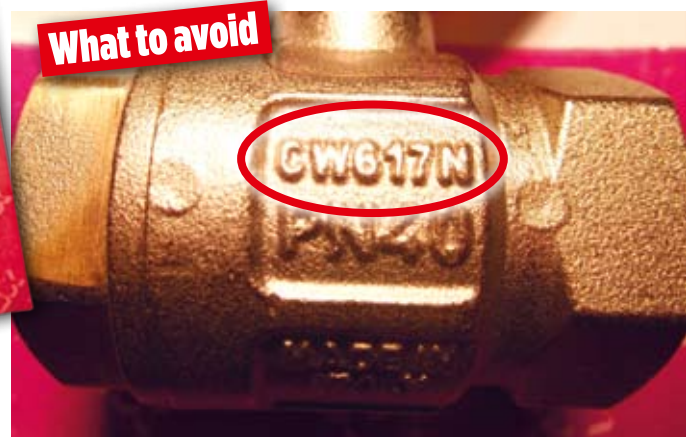
Brass valve removed from packaging and turned over to show marking
