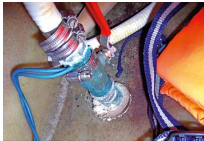
Time to panic! So much electrolytic action that the plywood backing pad is disintegrating due to electrochemical decay
