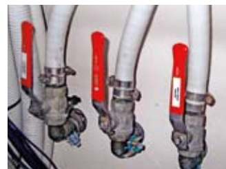
1998 boat built to RCD with non-marine brass valves
